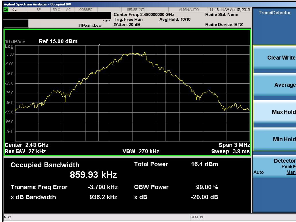
Plot 6-3. 20dB Bandwidth Plot (Bluetooth, 1Mbps – Ch. 78)
