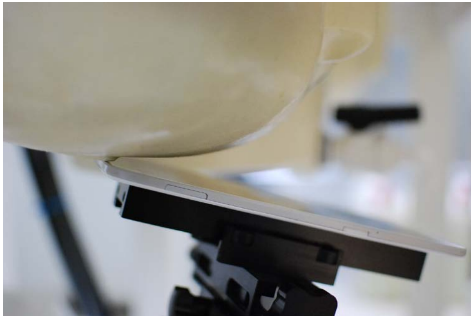
SAR Test Setup Photo 2 - Right Tilt
