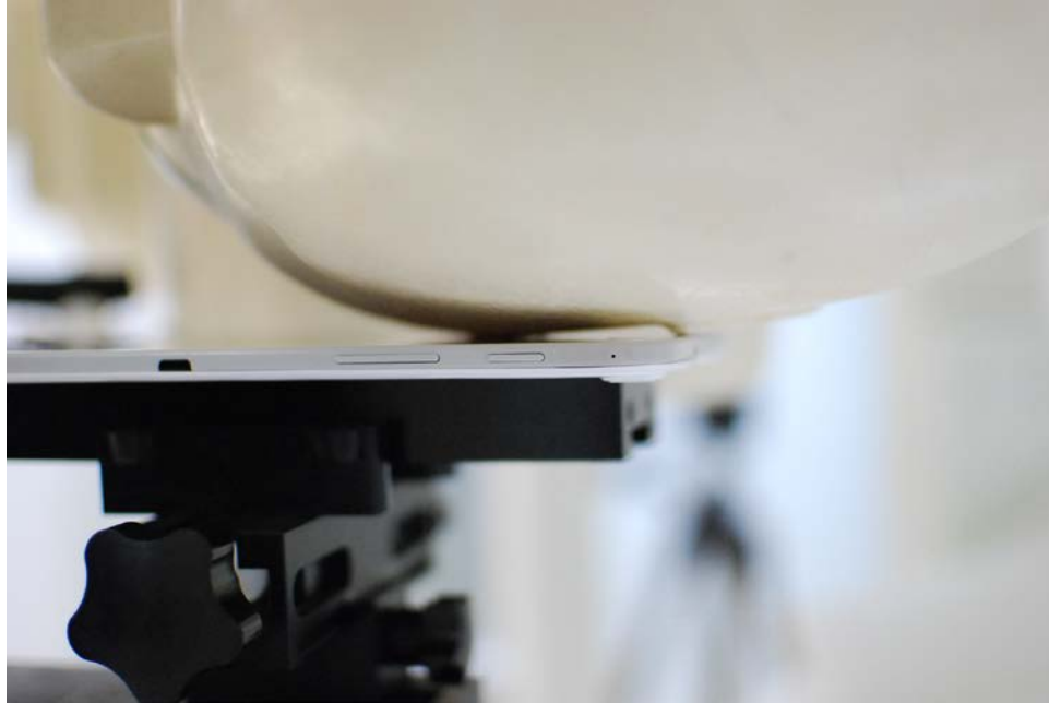
SAR Test Setup Photo 3 - Left Cheek
