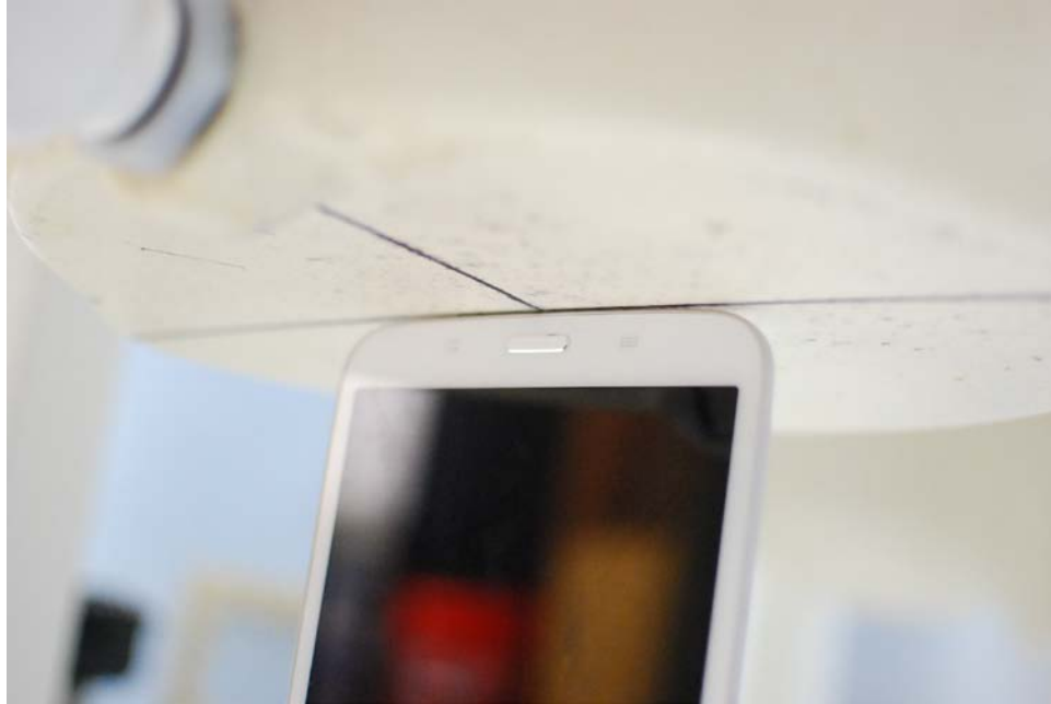
SAR Test Setup 9 - Bottom Edge at 0.0 cm
