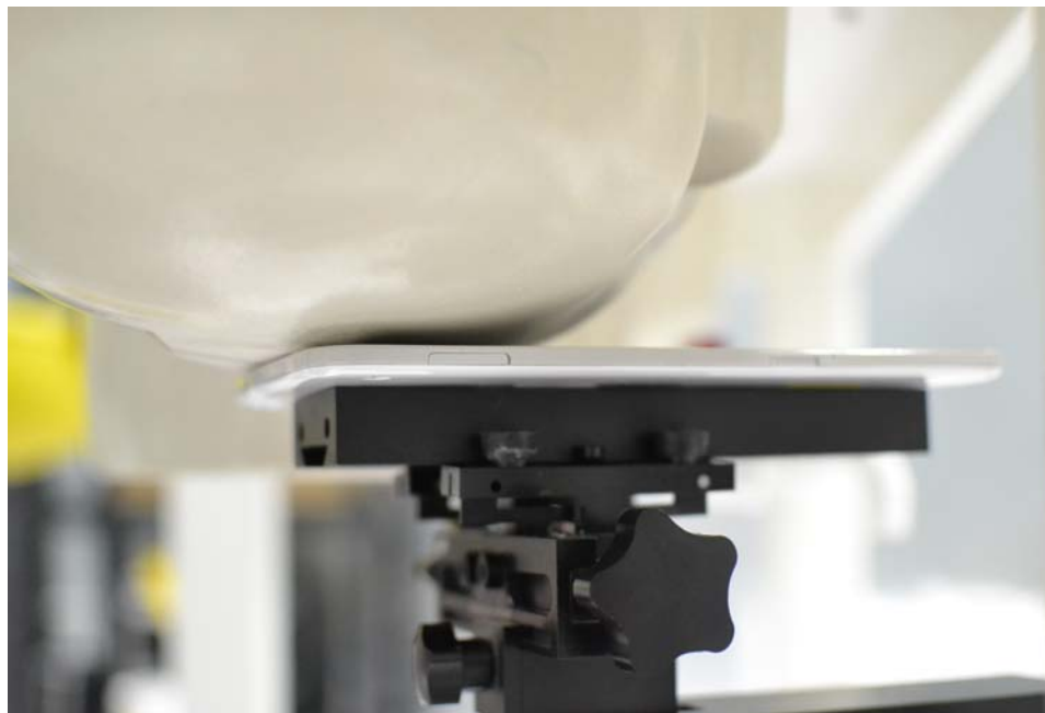
SAR Test Setup Photo 1: Right Cheek
