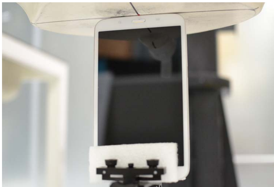
SAR Test Setup Photo 9: Bottom Edge at 0.0 cm
