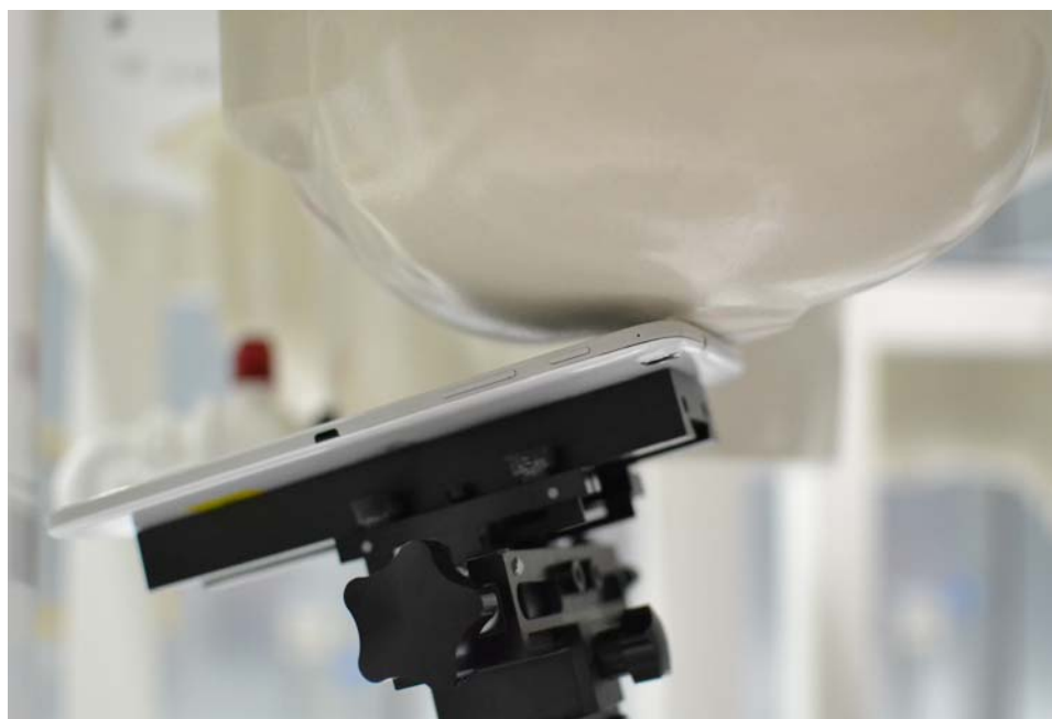
SAR Test Setup Photo 4: Left Tilt
