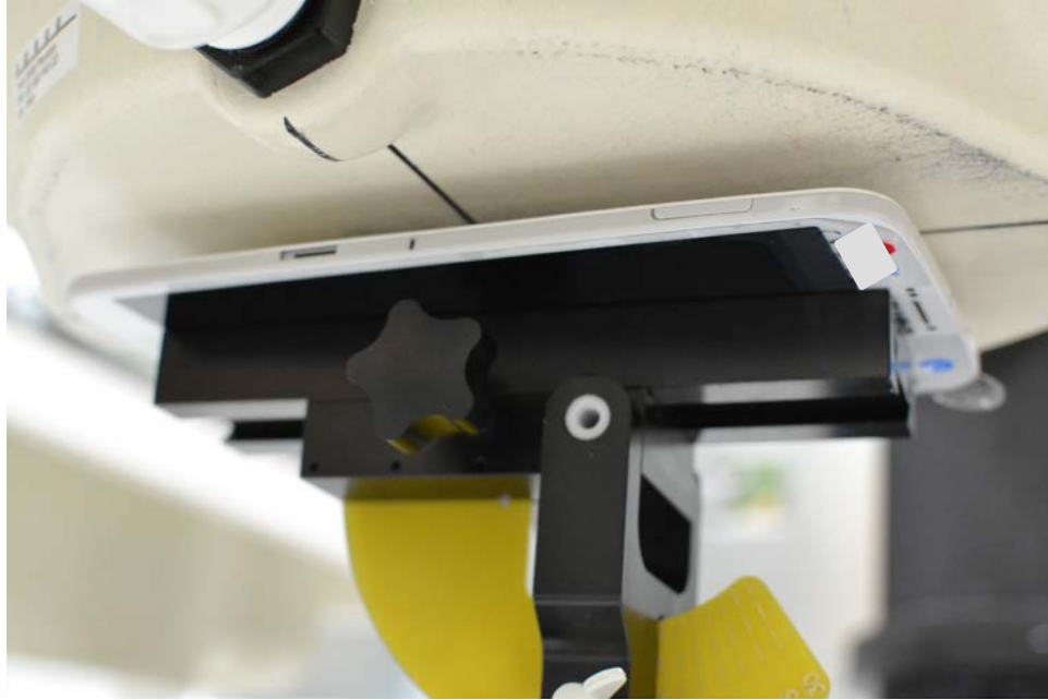
SAR Test Setup Photo 5: Back Side at 1.2 cm
