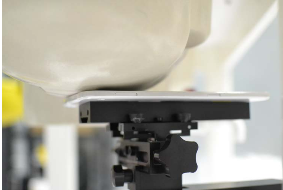
SAR Test Setup Photo 1: Right Cheek
