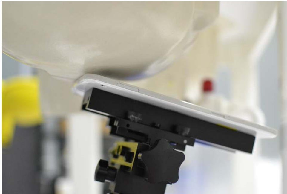
SAR Test Setup Photo 2: Right Tilt
