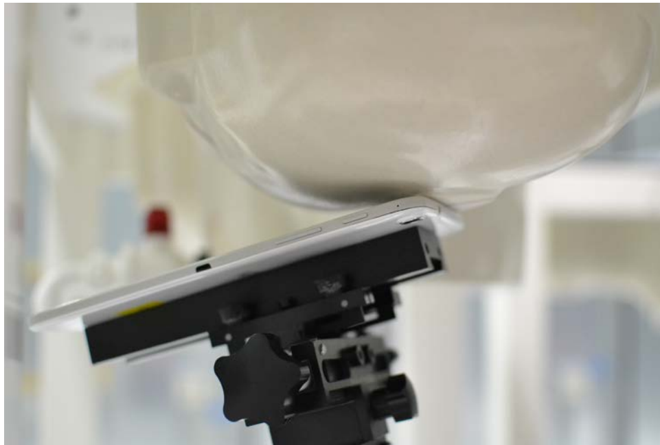
SAR Test Setup Photo 4: Left Tilt
