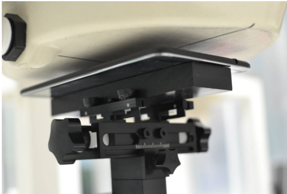
SAR Test Setup Photo 6 – Back side at 1.2 cm
