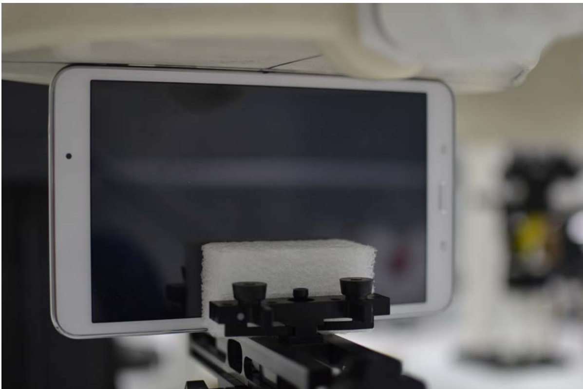
SAR Test Setup Photo 6 – Right Edge at 0 mm
