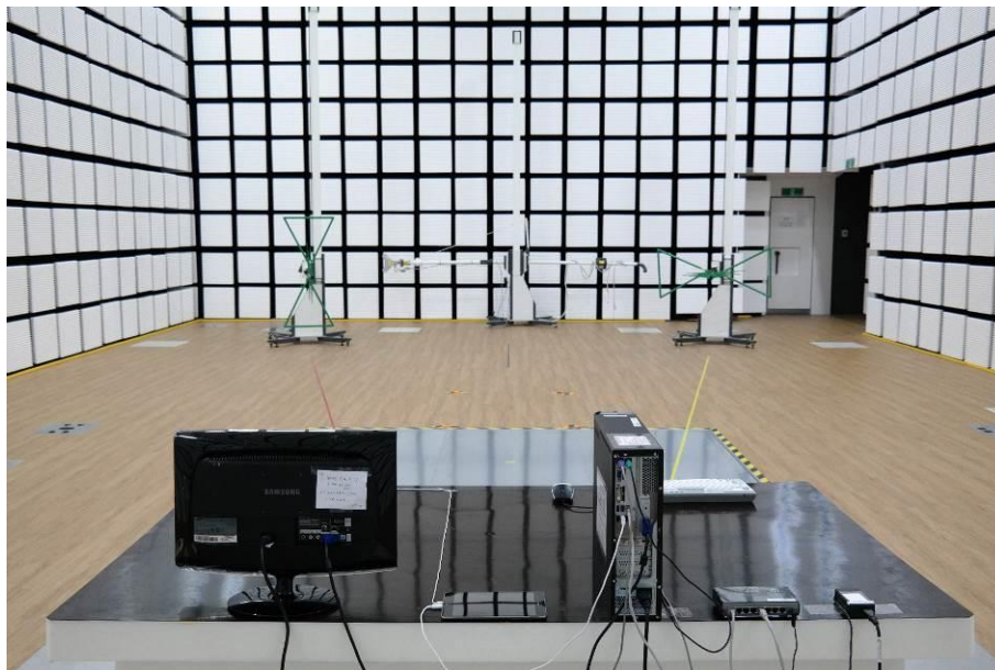
[ Radiated Disturbance for Below 1 GHz – Rear ]
