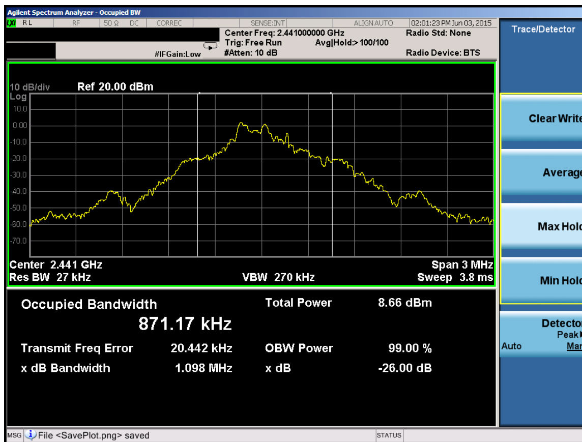
Plot 6-1. Occupied Bandwidth Plot (ANT+ – Ch. 39)
