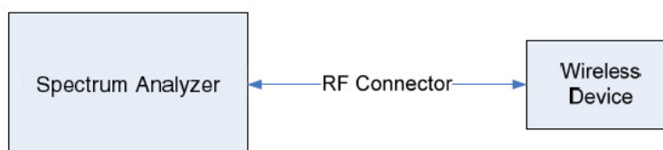
Figure 6-1. Test Instrument & Measurement Setup
