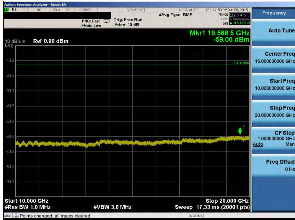
Plot 6-43. Conducted Spurious Plot (Band 4 – 1.4MHz QPSK – RB Size 1, RB Offset 0 – Mid Channel)
