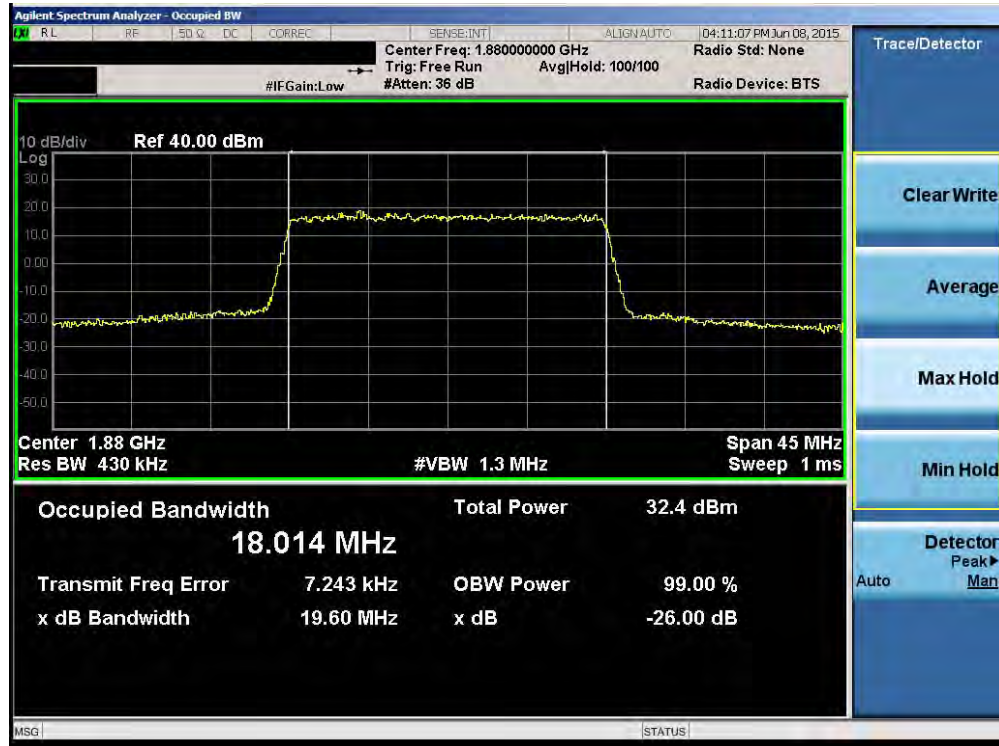
Plot 6-27. Occupied Bandwidth Plot (Band 2 – 20.0MHz QPSK – RB Size 100)
