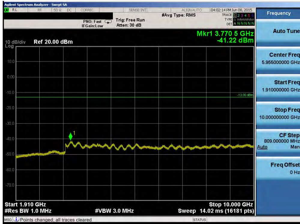
Plot 6-51. Conducted Spurious Plot (Band 2 – 15.0MHz QPSK – RB Size 1, RB Offset 0 – Mid Channel)
