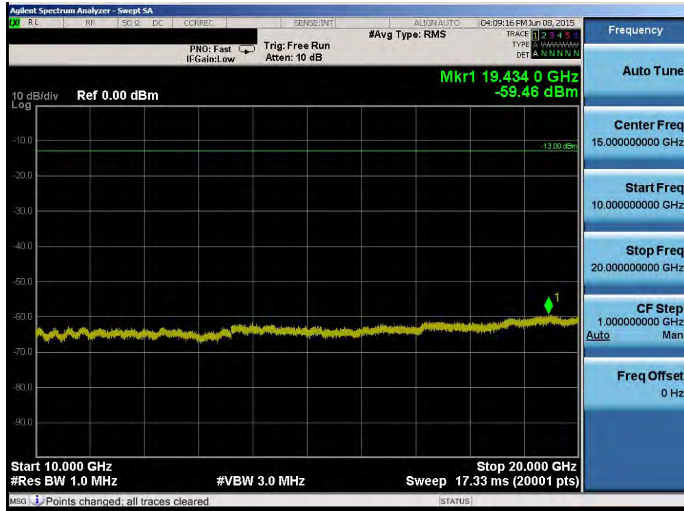
Plot 6-55. Conducted Spurious Plot (Band 2 – 15.0MHz QPSK – RB Size 1, RB Offset 0 – High Channel)
