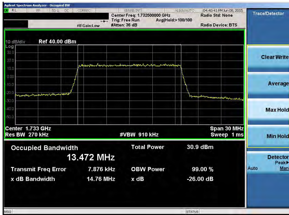
Plot 6-14. Occupied Bandwidth Plot (Band 4 – 15.0MHz 16-QAM – RB Size 75)
