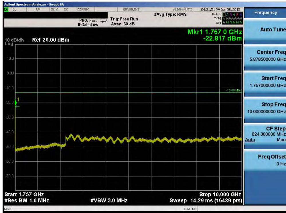
Plot 6-45. Conducted Spurious Plot (Band 4 – 1.4MHz QPSK – RB Size 1, RB Offset 0 – High Channel)
