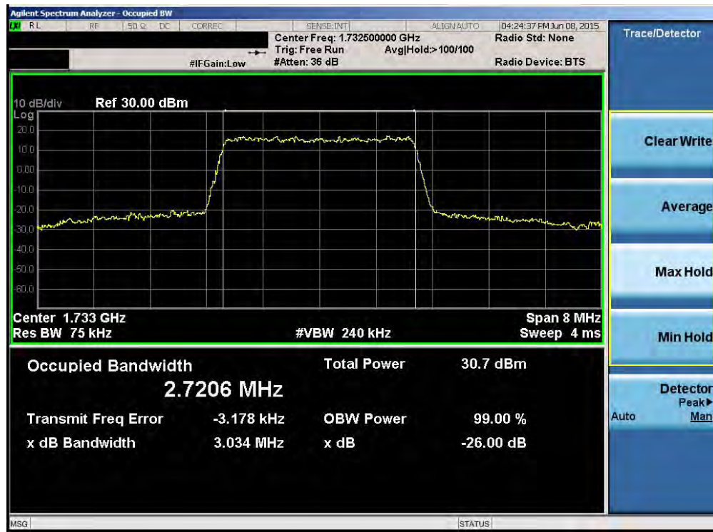
Plot 6-8. Occupied Bandwidth Plot (Band 4 – 3.0MHz 16-QAM – RB Size 15)
