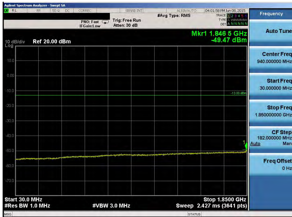
Plot 6-50. Conducted Spurious Plot (Band 2 – 15.0MHz QPSK – RB Size 1, RB Offset 0 – Mid Channel)
