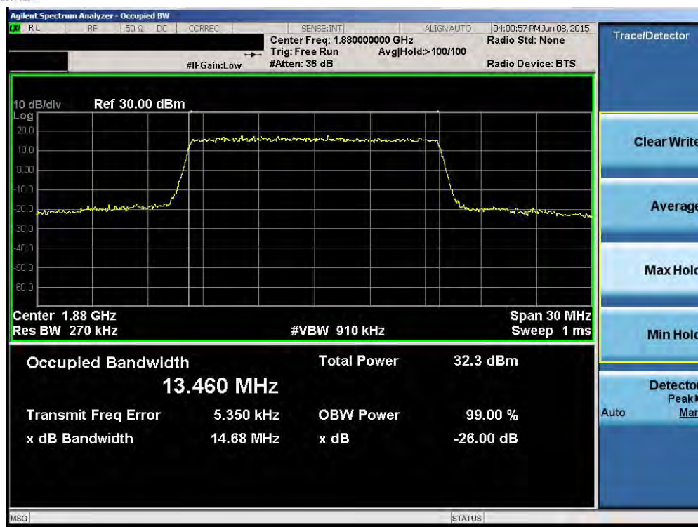
Plot 6-25. Occupied Bandwidth Plot (Band 2 – 15.0MHz QPSK – RB Size 75)
