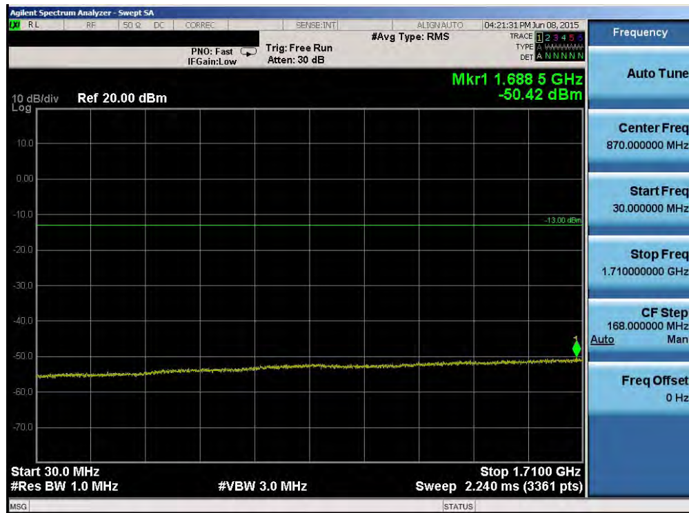
Plot 6-44. Conducted Spurious Plot (Band 4 – 1.4MHz QPSK – RB Size 1, RB Offset 0 – High Channel)
