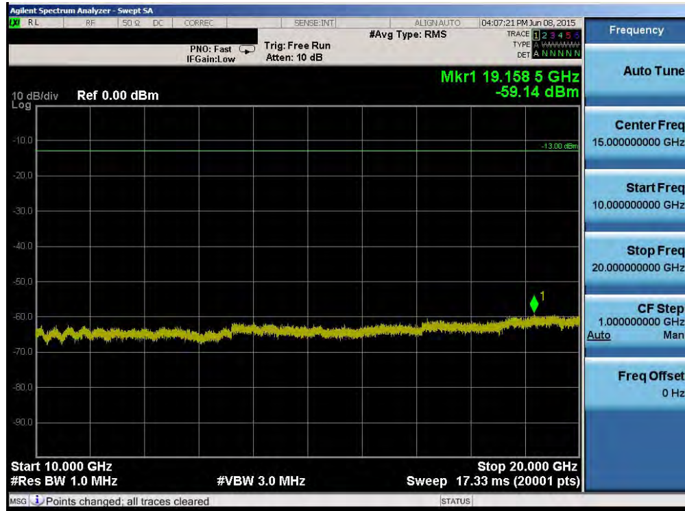
Plot 6-49. Conducted Spurious Plot (Band 2 – 15.0MHz QPSK – RB Size 1, RB Offset 0 – Low Channel)
