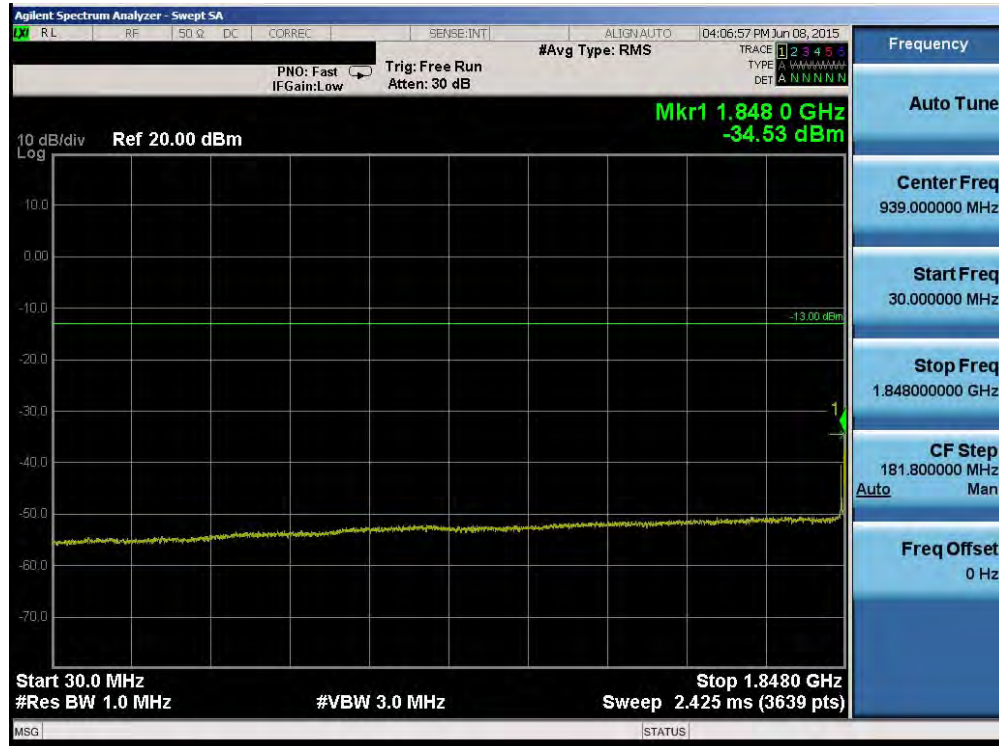
Plot 6-47. Conducted Spurious Plot (Band 2 – 15.0MHz QPSK – RB Size 1, RB Offset 0 – Low Channel)
