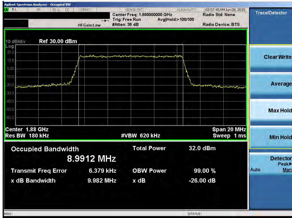
Plot 6-23. Occupied Bandwidth Plot (Band 2 – 10.0MHz QPSK – RB Size 50)
