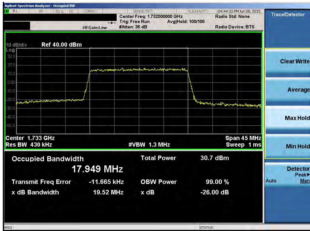
Plot 6-16. Occupied Bandwidth Plot (Band 4 – 20.0MHz 16-QAM – RB Size 100)
