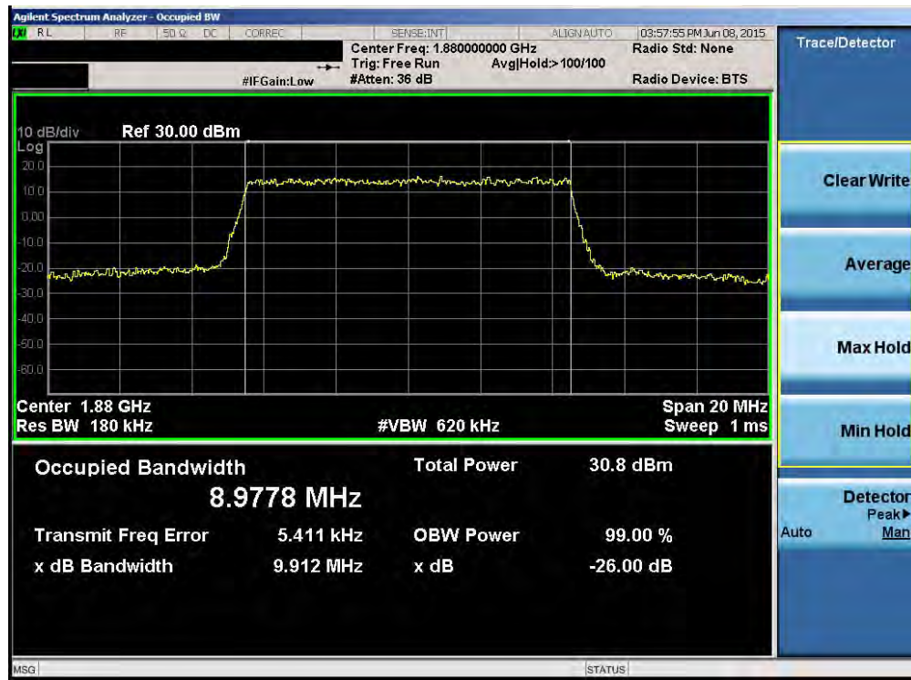
Plot 6-24. Occupied Bandwidth Plot (Band 2 – 10.0MHz 16-QAM – RB Size 50)
