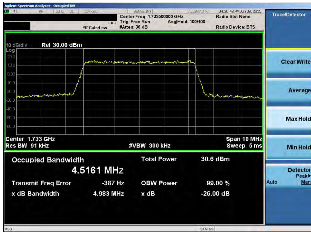
Plot 6-10. Occupied Bandwidth Plot (Band 4 – 5.0MHz 16-QAM – RB Size 25)
