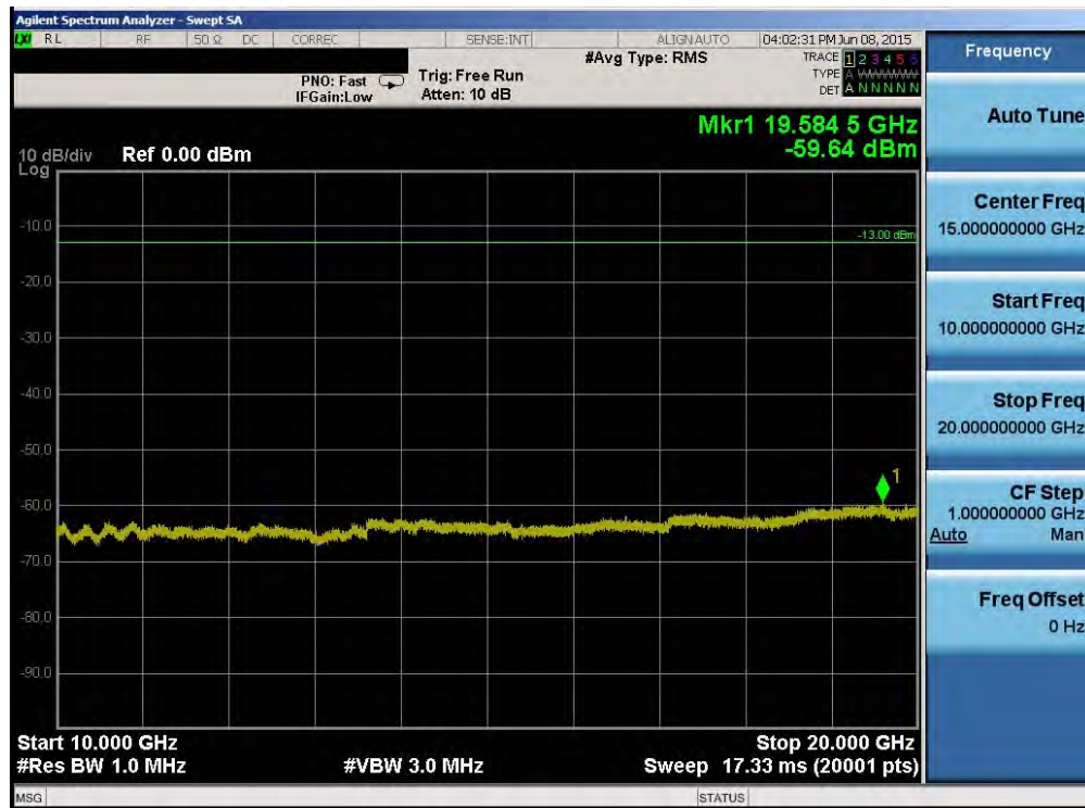
Plot 6-52. Conducted Spurious Plot (Band 2 – 15.0MHz QPSK – RB Size 1, RB Offset 0 – Mid Channel)
