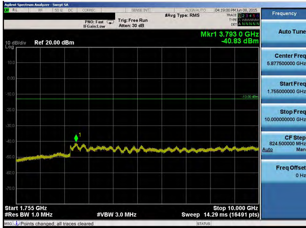
Plot 6-39. Conducted Spurious Plot (Band 4 – 1.4MHz QPSK – RB Size 1, RB Offset 0 – Low Channel)
