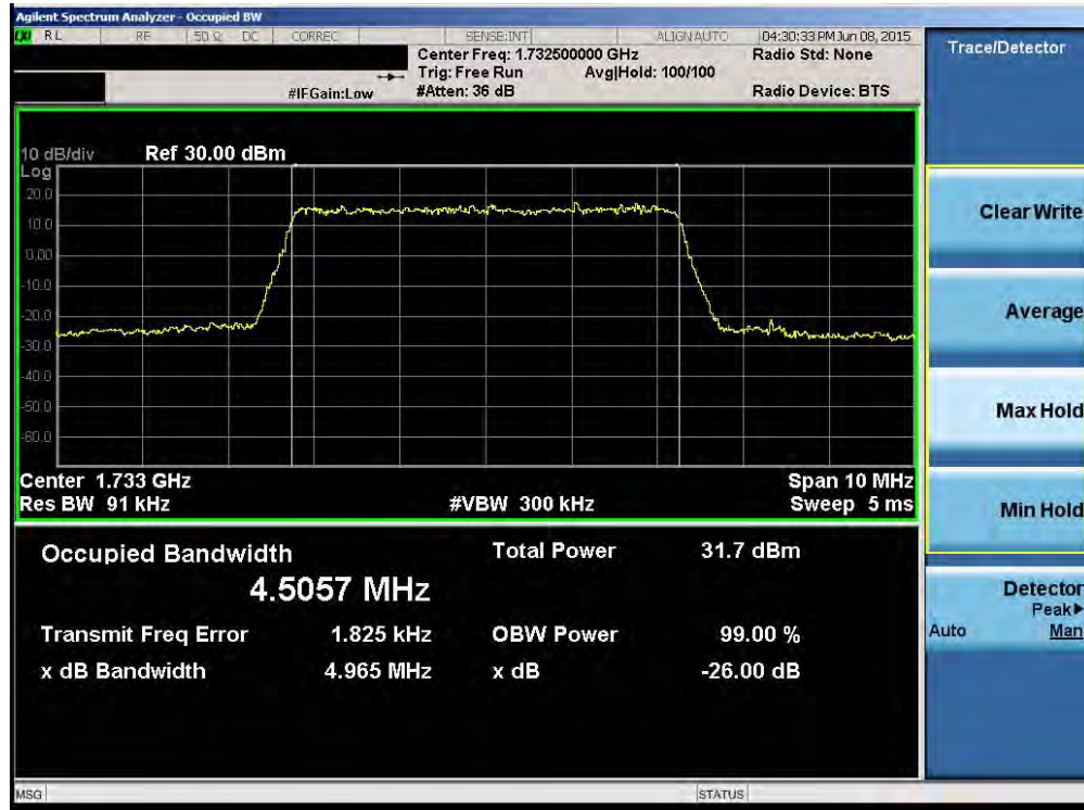
Plot 6-9. Occupied Bandwidth Plot (Band 4 – 5.0MHz QPSK – RB Size 25)
