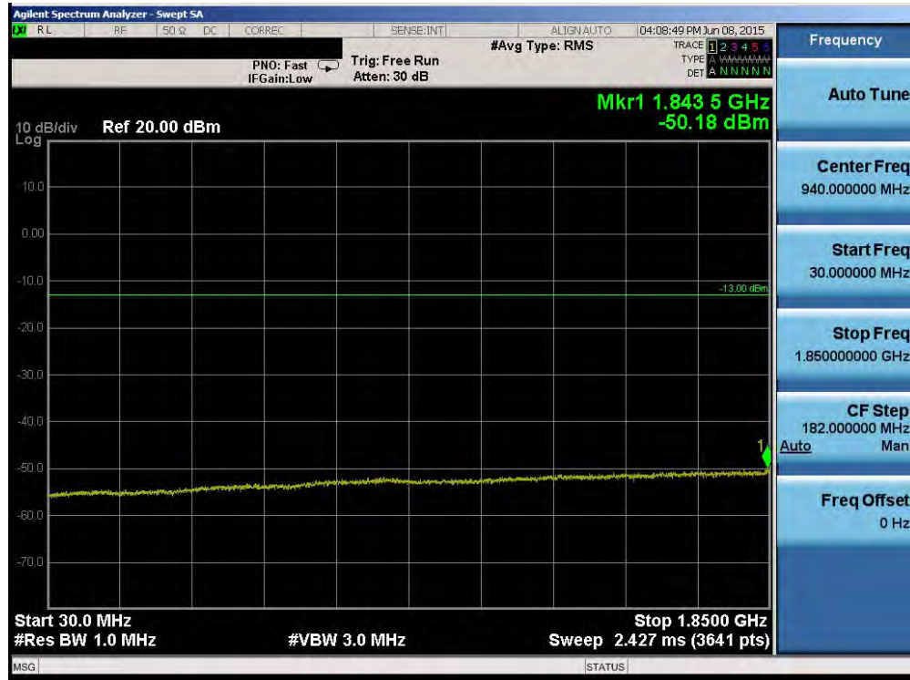
Plot 6-53. Conducted Spurious Plot (Band 2 – 15.0MHz QPSK – RB Size 1, RB Offset 0 – High Channel)
