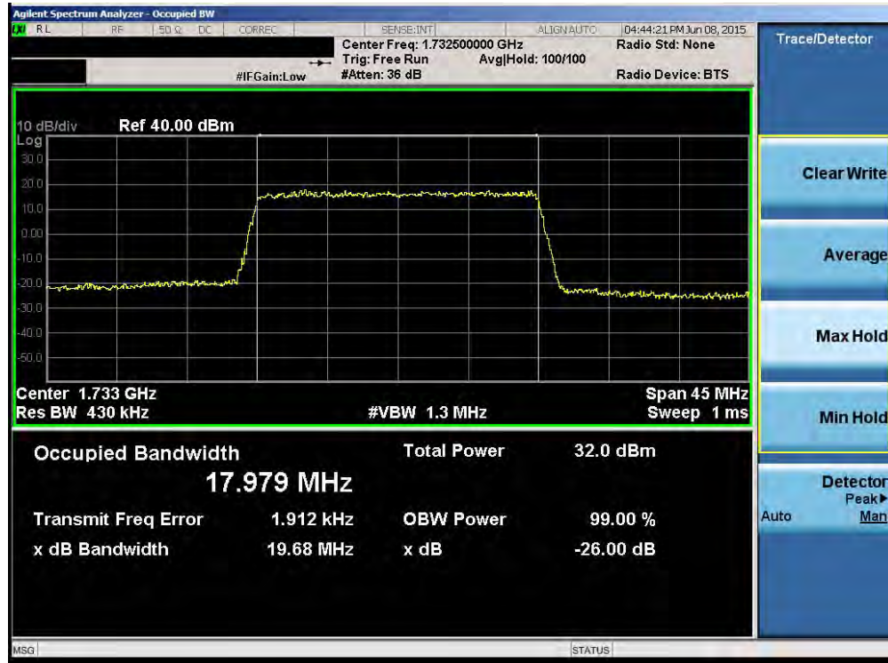
Plot 6-15. Occupied Bandwidth Plot (Band 4 – 20.0MHz QPSK – RB Size 100)
