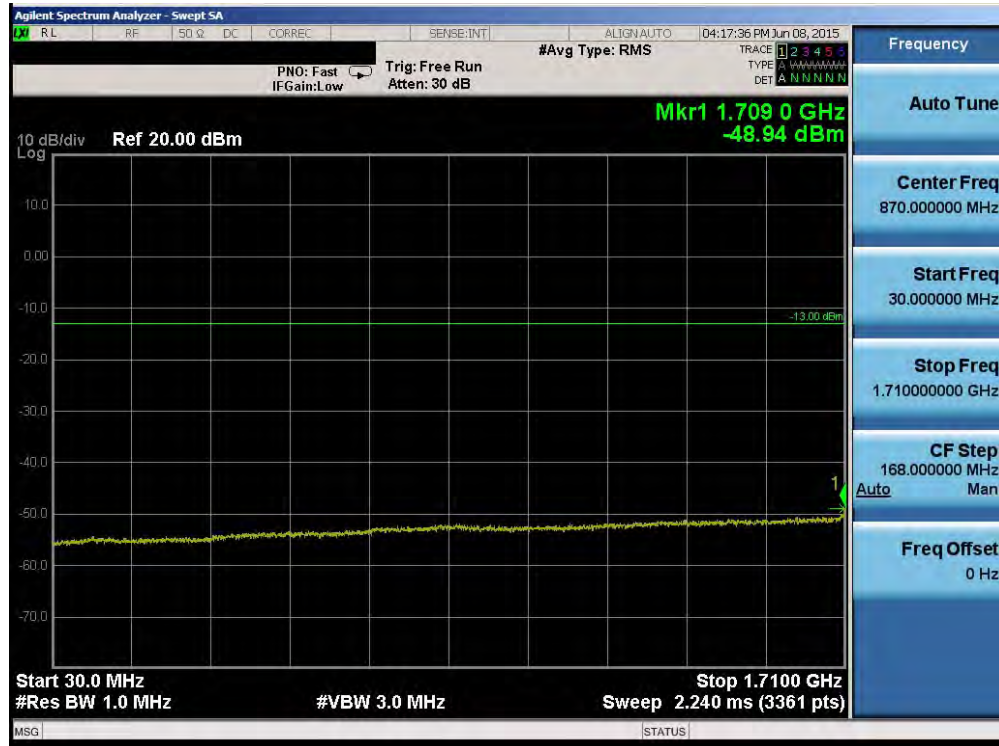
Plot 6-41. Conducted Spurious Plot (Band 4 – 1.4MHz QPSK – RB Size 1, RB Offset 0 – Mid Channel)
