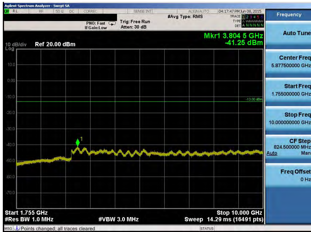
Plot 6-42. Conducted Spurious Plot (Band 4 – 1.4MHz QPSK – RB Size 1, RB Offset 0 – Mid Channel)
