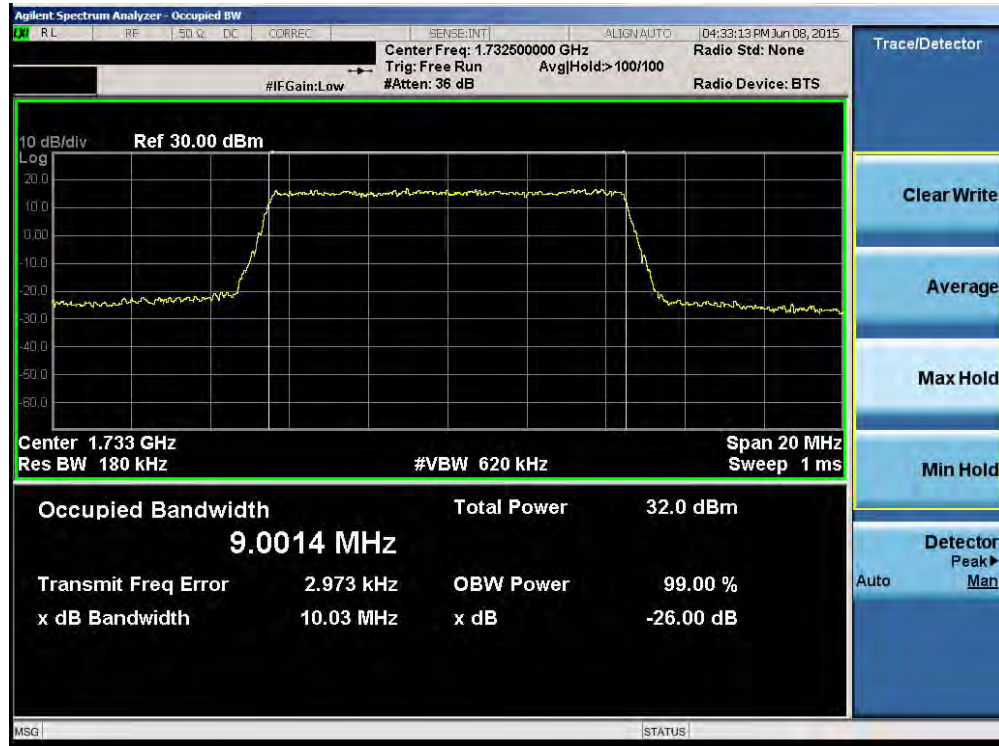
Plot 6-11. Occupied Bandwidth Plot (Band 4 – 10.0MHz QPSK – RB Size 50)
