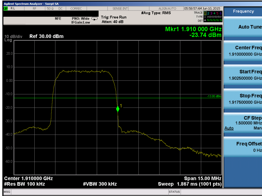
Plot 6-39. Band Edge Plot (PCS WCDMA Mode – Ch. 9538)
