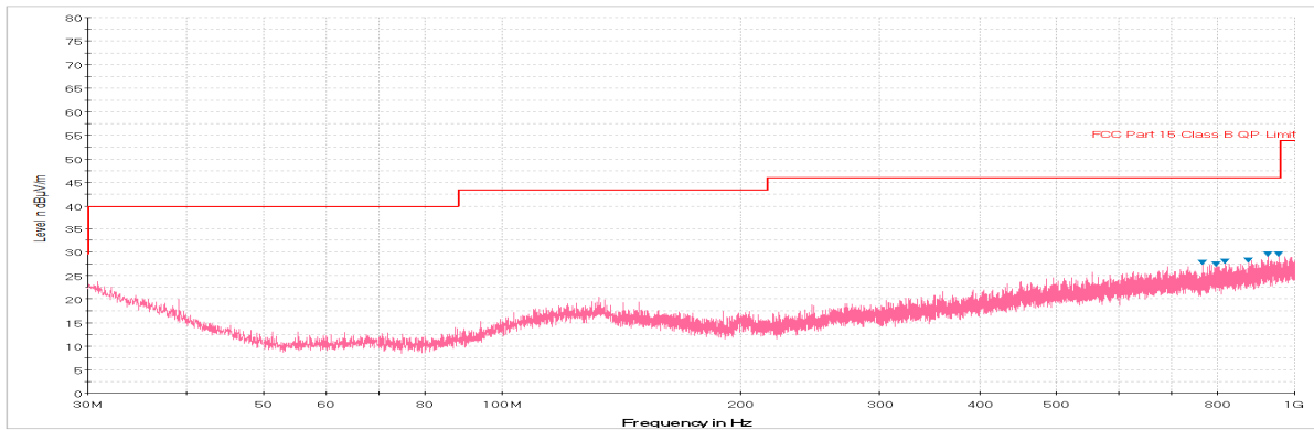
Plot 6-91. Radiated Spurious Plot below 1GHz (802.11a – U3 Ch. 157, Ant. Pol. H)
