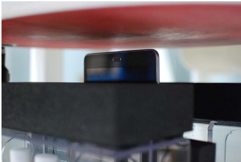
SAR Test Setup Photo 6: Bottom Edge at 1.8 cm
