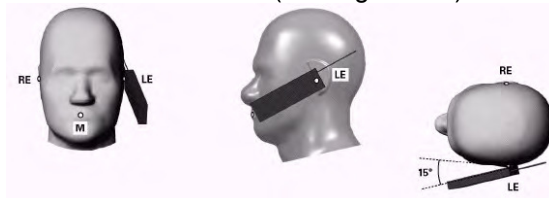
Figure 7-2 Front, Side and Top View of Ear/15° Tilt Position
