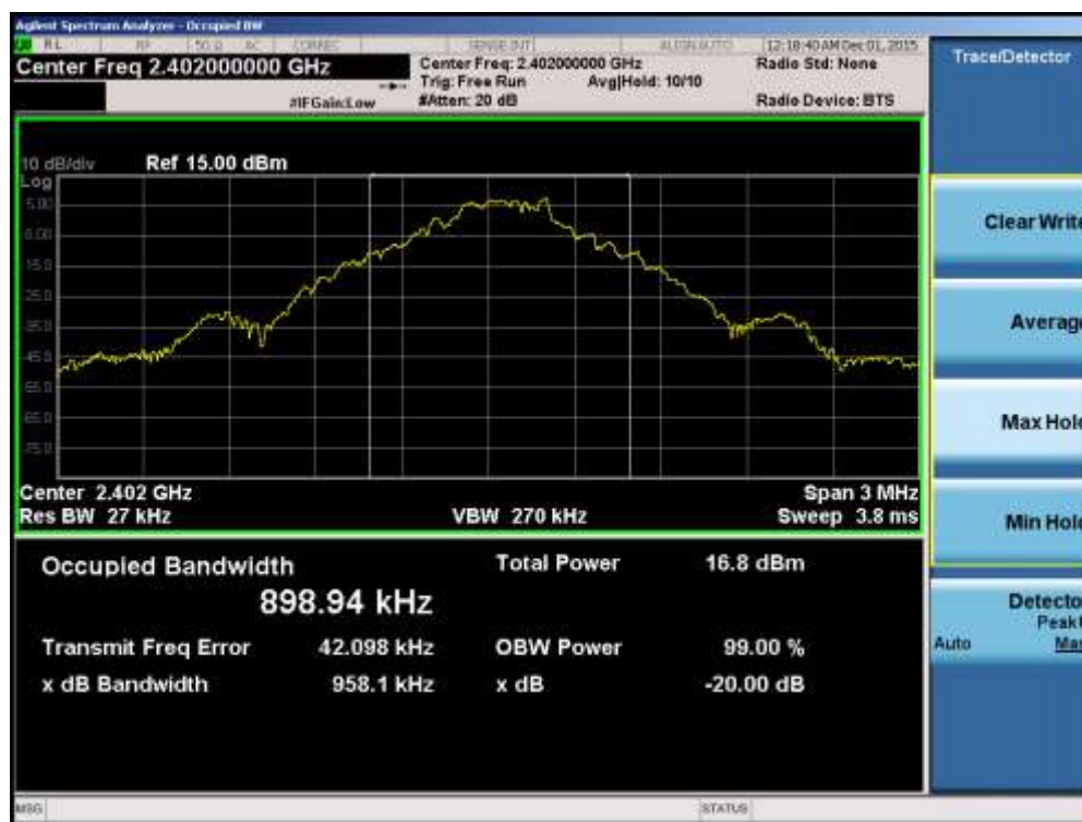
Plot 7-1. 20dB Bandwidth Plot (Bluetooth, 1Mbps – Ch. 0)
