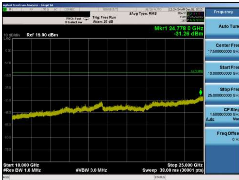
Plot 7-41. Conducted Spurious Plot (Bluetooth, 1Mbps – Ch. 78)
