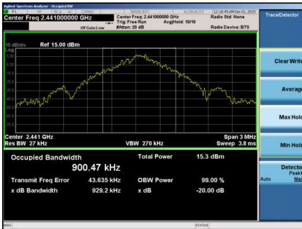
Plot 7-2. 20dB Bandwidth Plot (Bluetooth, 1Mbps – Ch. 39)
