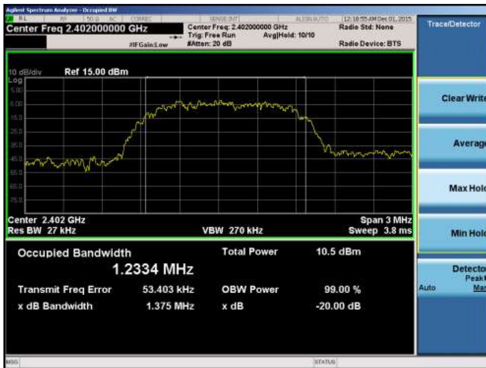
Plot 7-4. 20dB Bandwidth Plot (Bluetooth, 2Mbps – Ch. 0)
