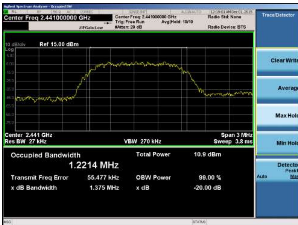
Plot 7-5. 20dB Bandwidth Plot (Bluetooth, 2Mbps – Ch. 39)
