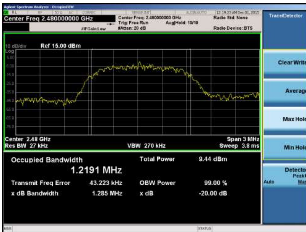
Plot 7-9. 20dB Bandwidth Plot (Bluetooth, 3Mbps – Ch. 78)
