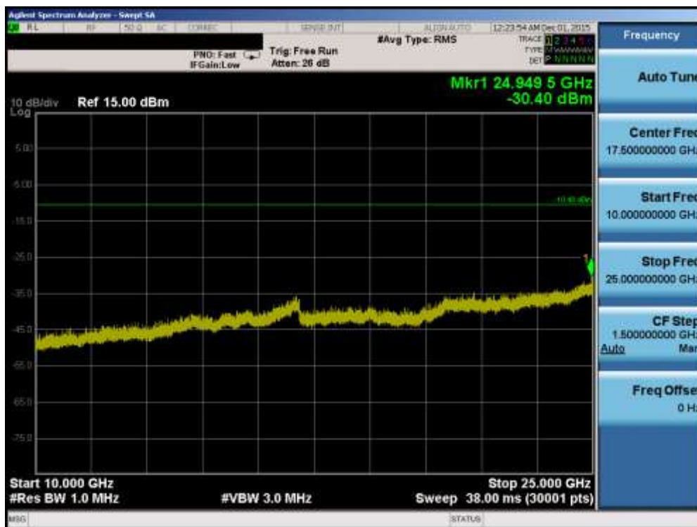
Plot 7-39. Conducted Spurious Plot (Bluetooth, 1Mbps – Ch. 39)
