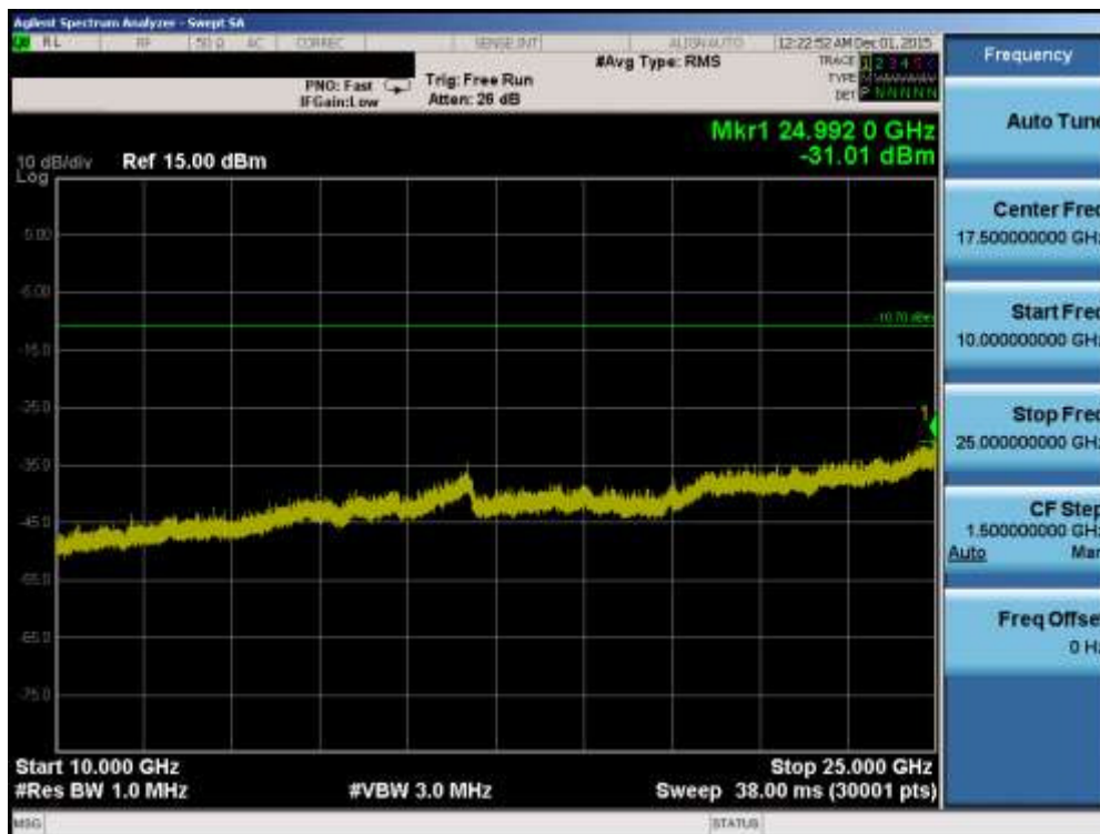
Plot 7-37. Conducted Spurious Plot (Bluetooth, 1Mbps – Ch. 0)
