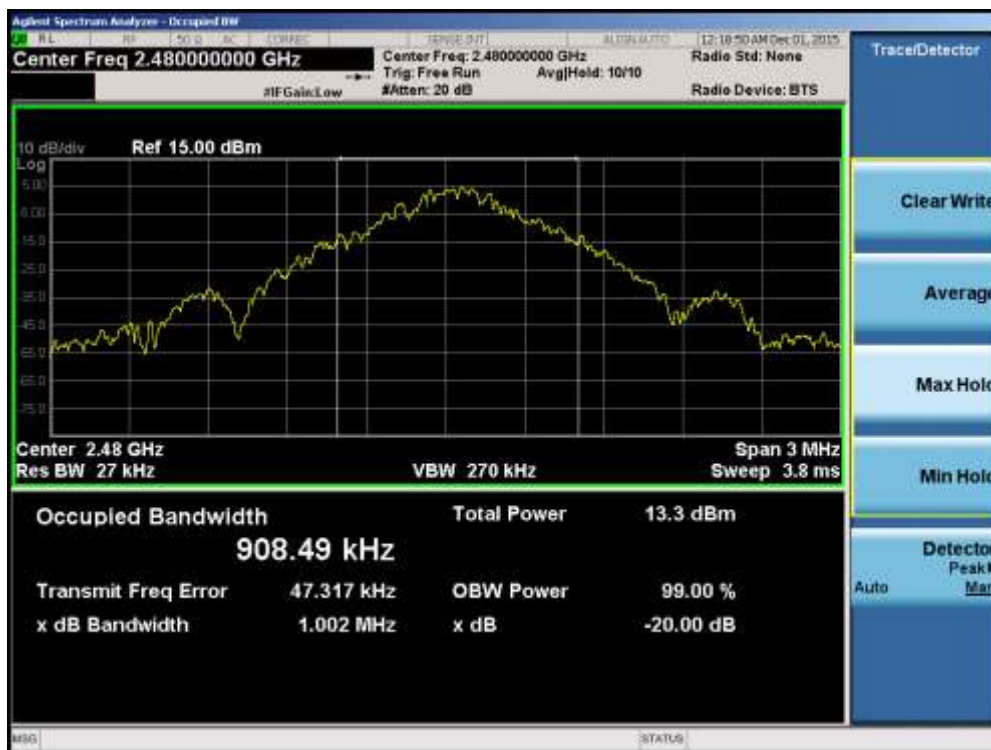
Plot 7-3. 20dB Bandwidth Plot (Bluetooth, 1Mbps – Ch. 78)
