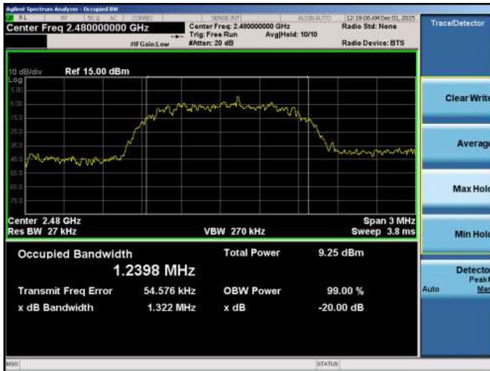
Plot 7-6. 20dB Bandwidth Plot (Bluetooth, 2Mbps – Ch. 78)
