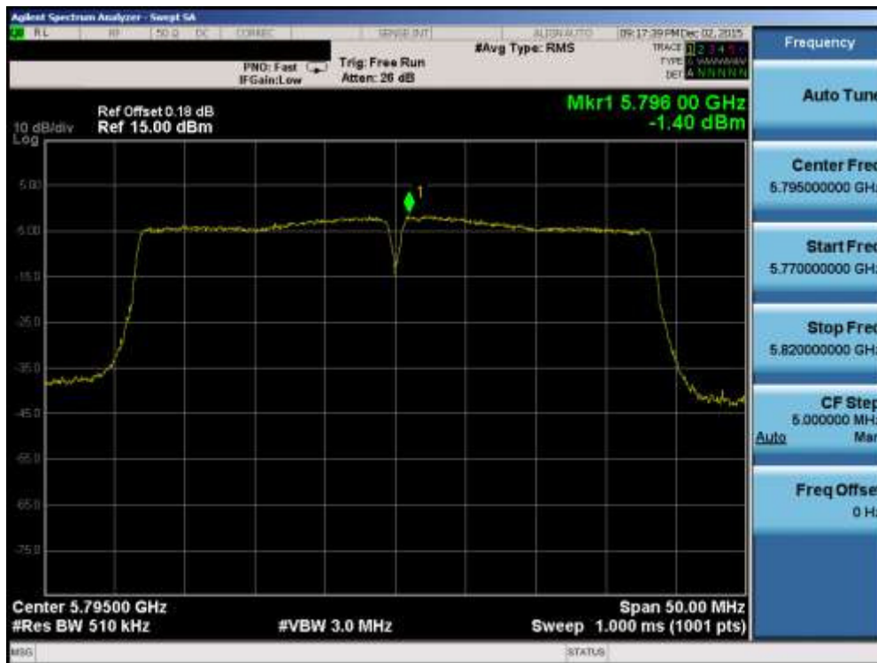
Plot 7-66. Power Spectral Density Plot (40MHz BW 802.11n (UNII Band 3) – Ch. 159)
