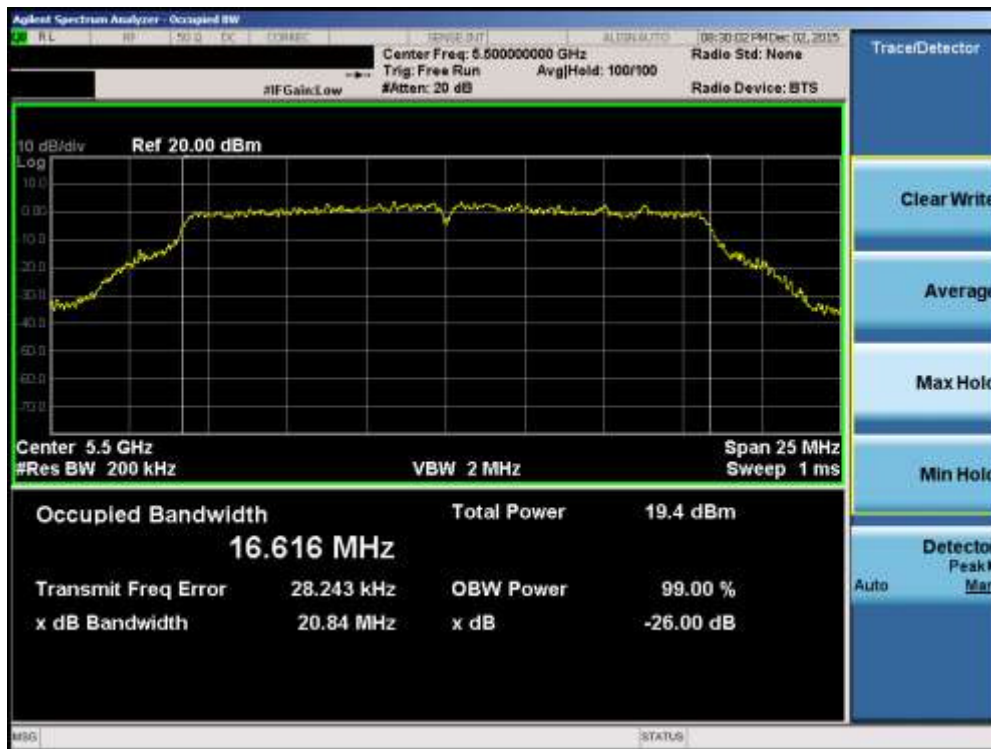
Plot 7-17. 26dB Bandwidth Plot (802.11a (UNII Band 2C) – Ch. 100)
