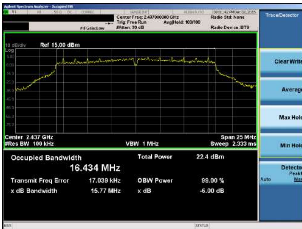
Plot 7-5. 6dB Bandwidth Plot (802.11g – Ch. 6)
