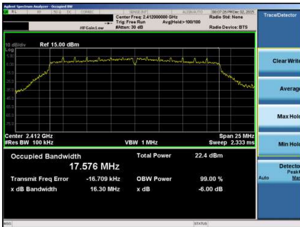
Plot 7-7. 6dB Bandwidth Plot (802.11n (2.4GHz) – Ch. 1)
