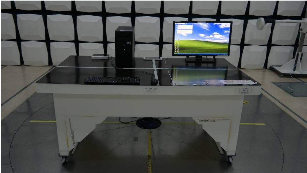
[ Radiated Disturbance for Below 1 GHz – Front ]
