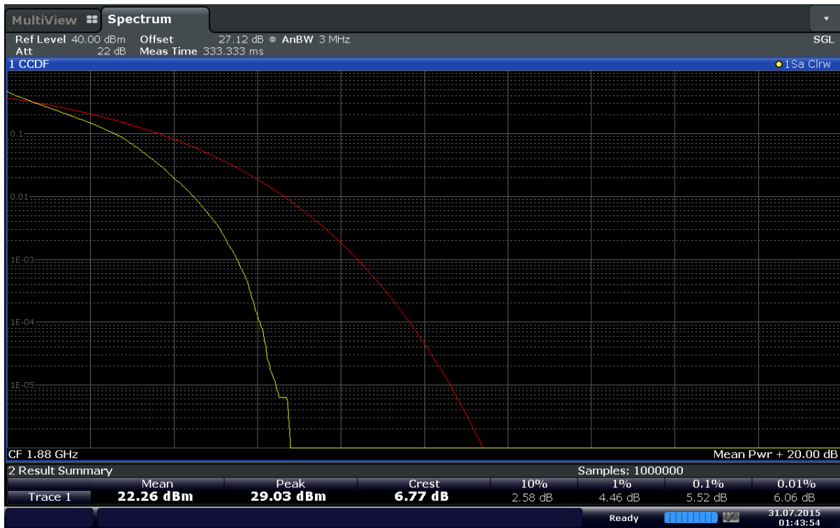
Plot 6-115. Peak-Average Ratio Plot (Band 2 – 3.0MHz QPSK - RB Size 15)
