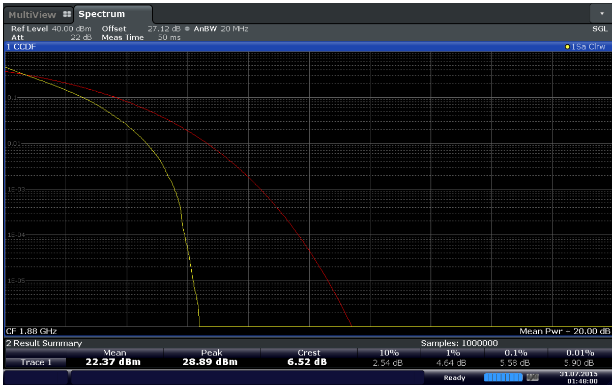
Plot 6-121. Peak-Average Ratio Plot (Band 2 – 15.0MHz QPSK - RB Size 75)
