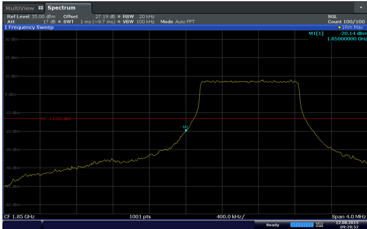
Plot 6-69. Lower Band Edge Plot (Band2 – 1.4MHz – QPSK – RB Size 6)
