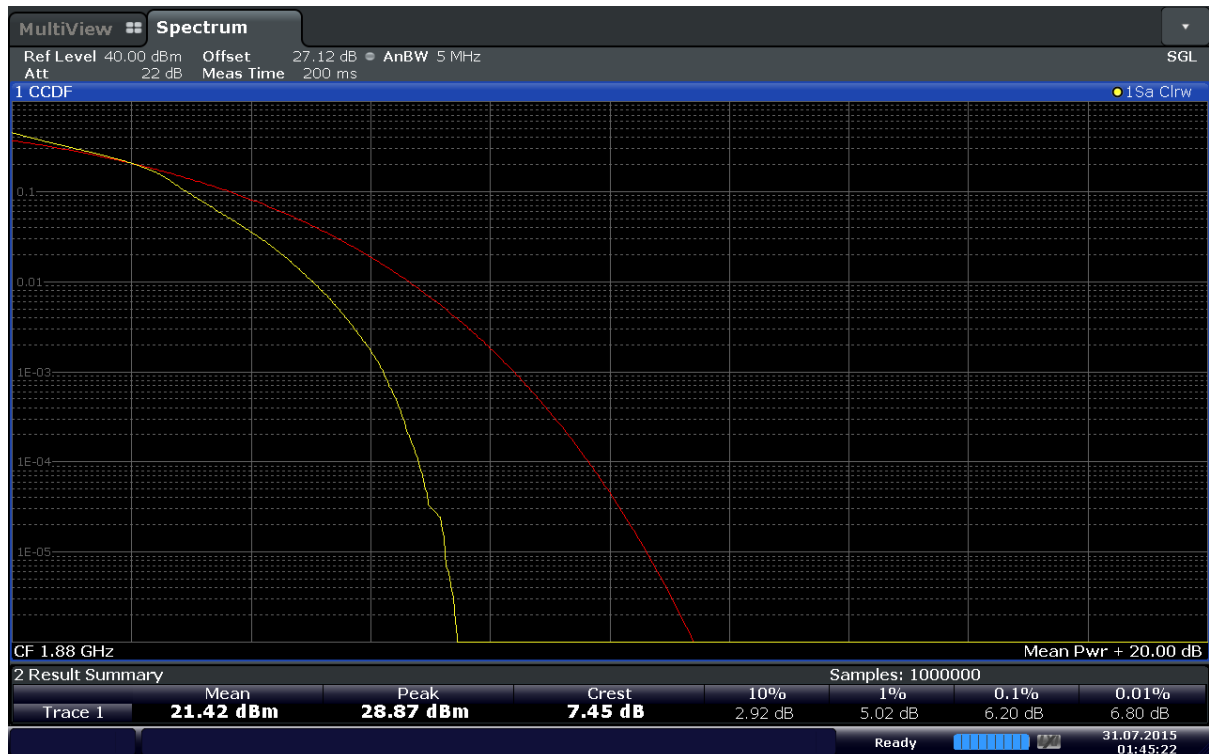
Plot 6-118. Peak-Average Ratio Plot (Band 2 – 5.0MHz 16QAM - RB Size 25)
