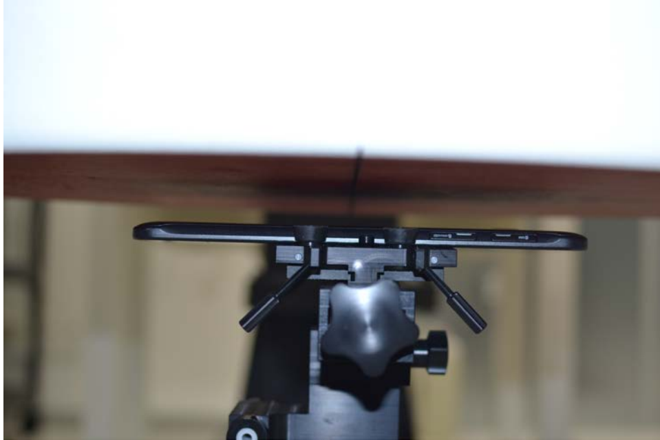
SAR Test Setup Photo 1: Back Side at 1.7 cm
