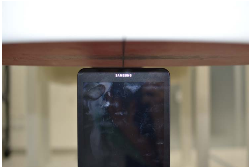
SAR Test Setup Photo 4: Top Edge at 1.3 cm
