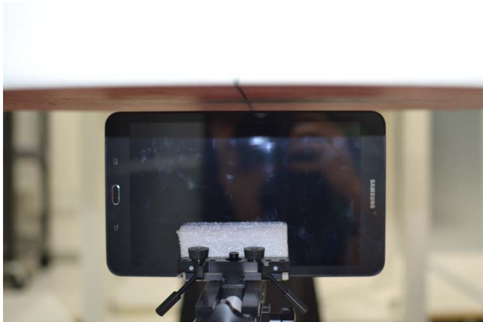
SAR Test Setup Photo 7: Left Edge at 0.6 cm
