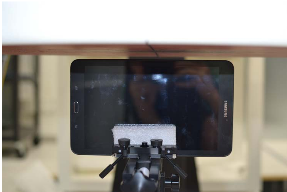
SAR Test Setup Photo 6: Left Edge at 0.9 cm
