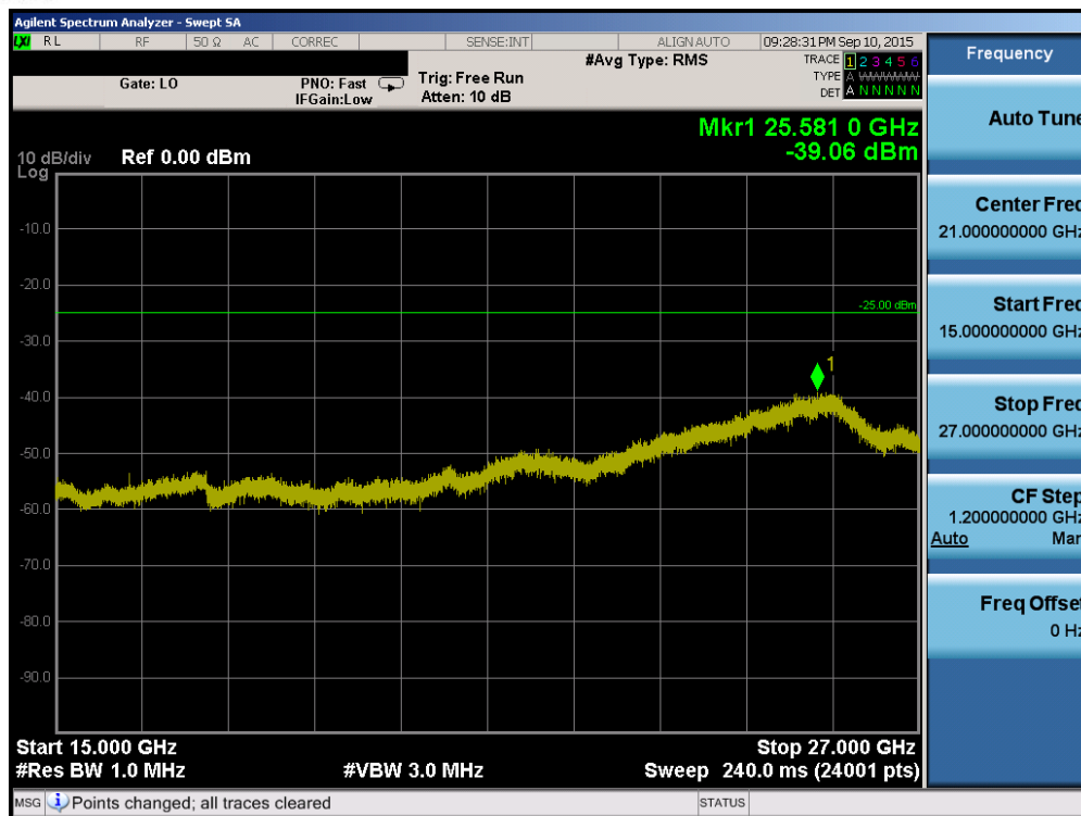
Plot 6-95. Conducted Spurious Plot (Band 41 – 20.0MHz QPSK – RB Size 1, RB Offset 0 – High Channel)
