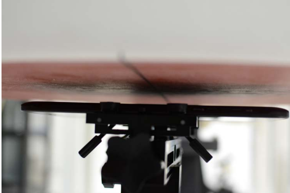
SAR Test Setup Photo 1: Back Side at 1.5 cm
