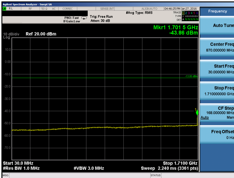
Plot 7-48. Conducted Spurious Plot (Band 4 – 20.0MHz QPSK – RB Size 1, RB Offset 0 – High Channel)
