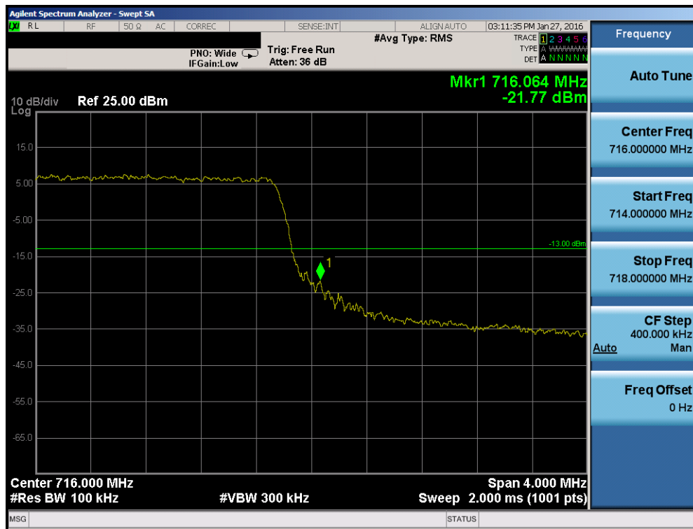
Plot 7-65. Upper Band Edge Plot (Band 12 – 5.0MHz QPSK – RB Size 25)
