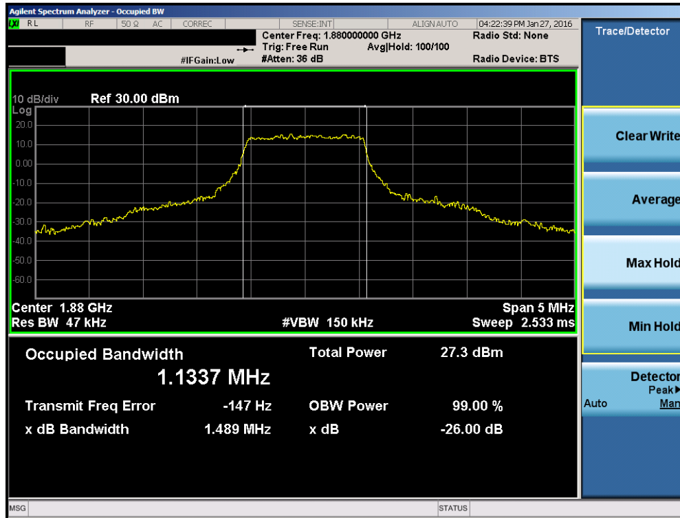
Plot 7-21. Occupied Bandwidth Plot (Band 2 – 1.4MHz QPSK – RB Size 6)
