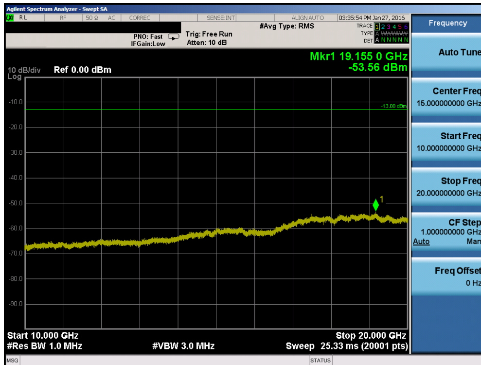
Plot 7-56. Conducted Spurious Plot (Band 2 – 20.0MHz QPSK – RB Size 1, RB Offset 0 – Mid Channel)
