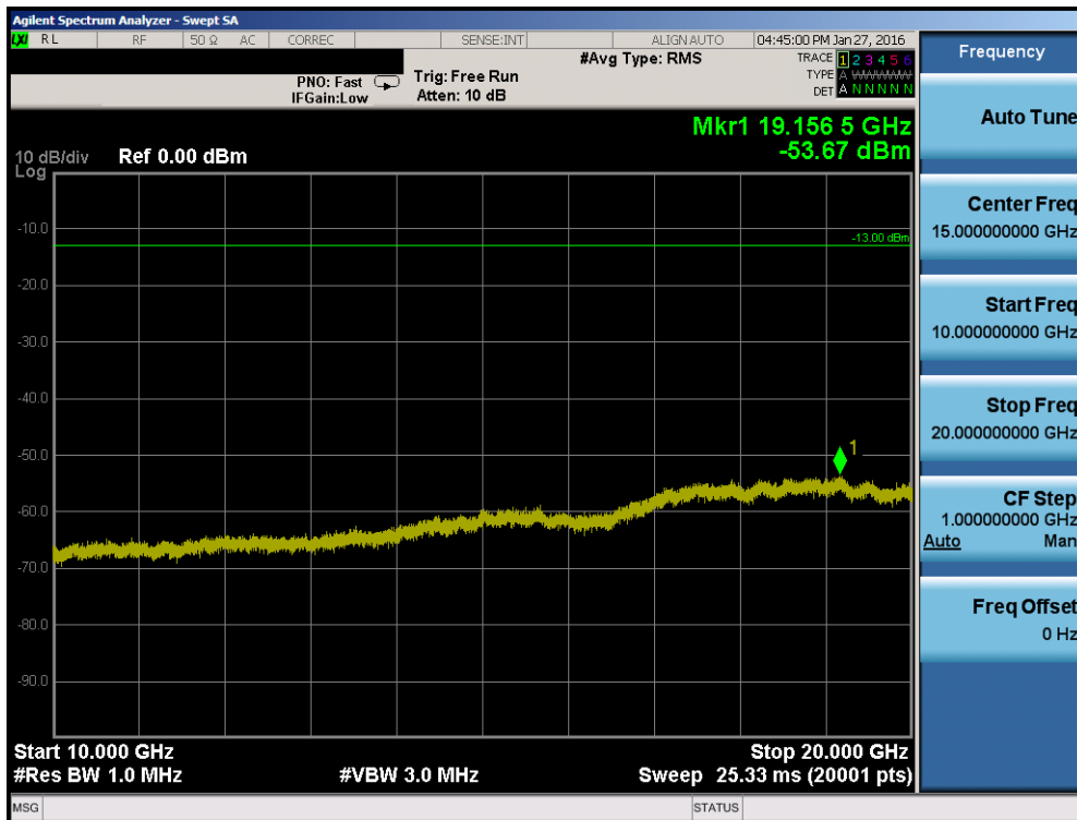
Plot 7-44. Conducted Spurious Plot (Band 4 – 20.0MHz QPSK – RB Size 1, RB Offset 0 – Low Channel)
