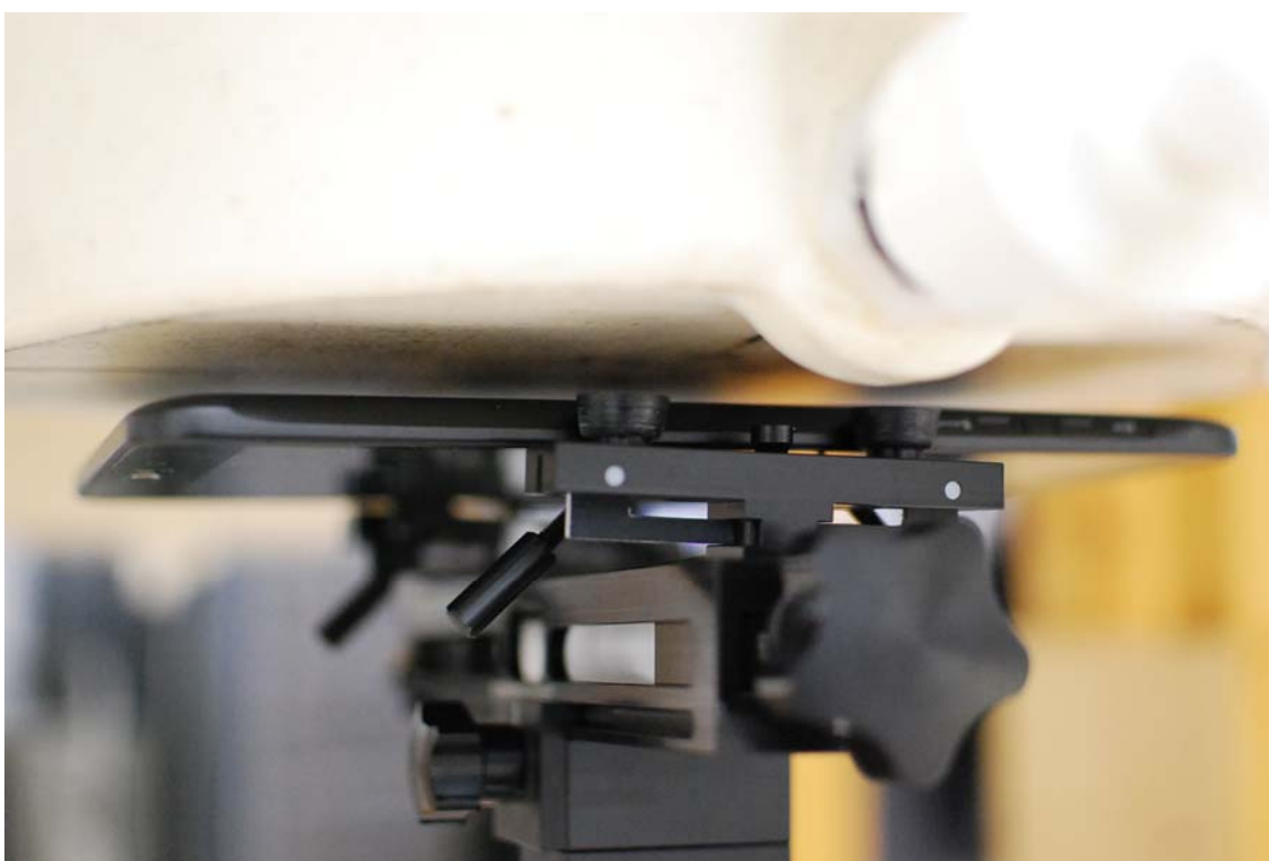
SAR Test Setup Photo 1: Back Side at 12 mm
