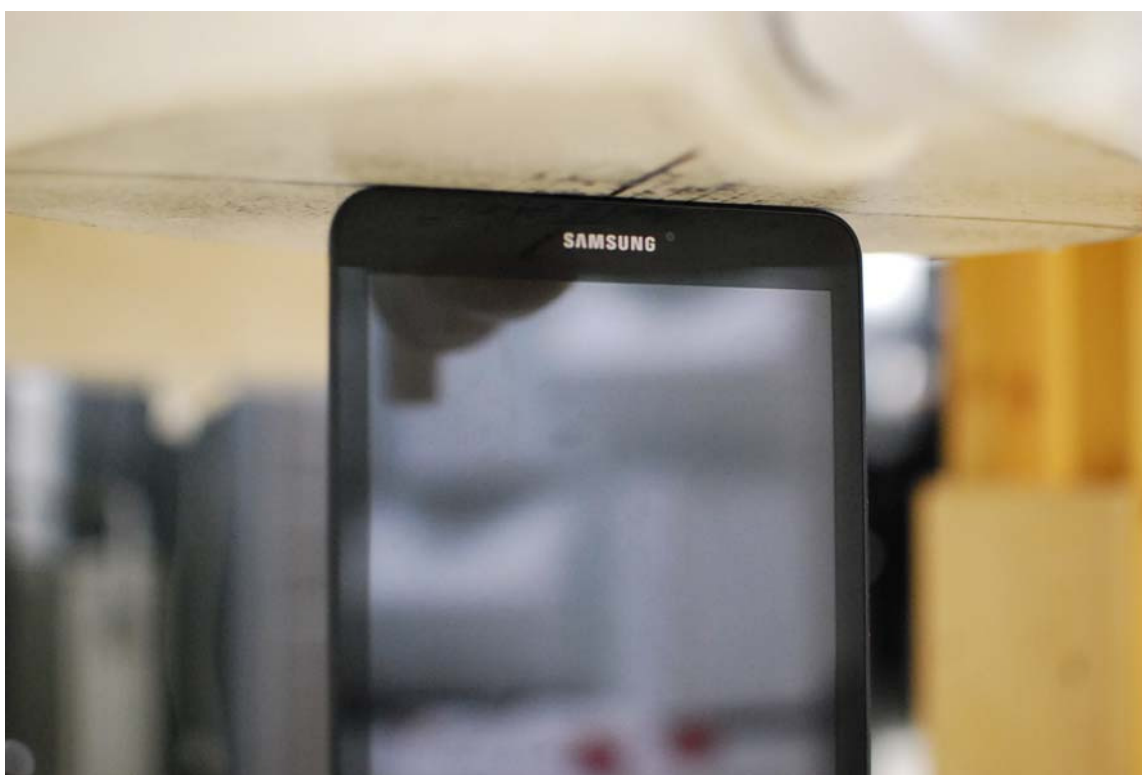
SAR Test Setup Photo 1: Top Edge at 0 mm
