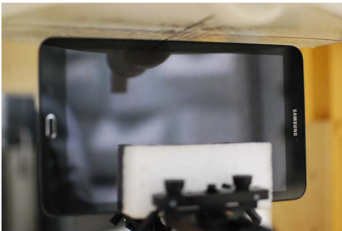
SAR Test Setup Photo 1: Left Edge at 6 mm
