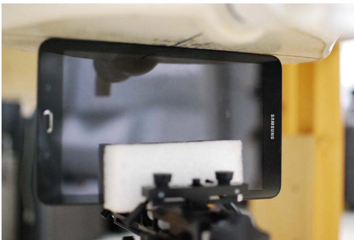
SAR Test Setup Photo 1: Left Edge at 0 mm
