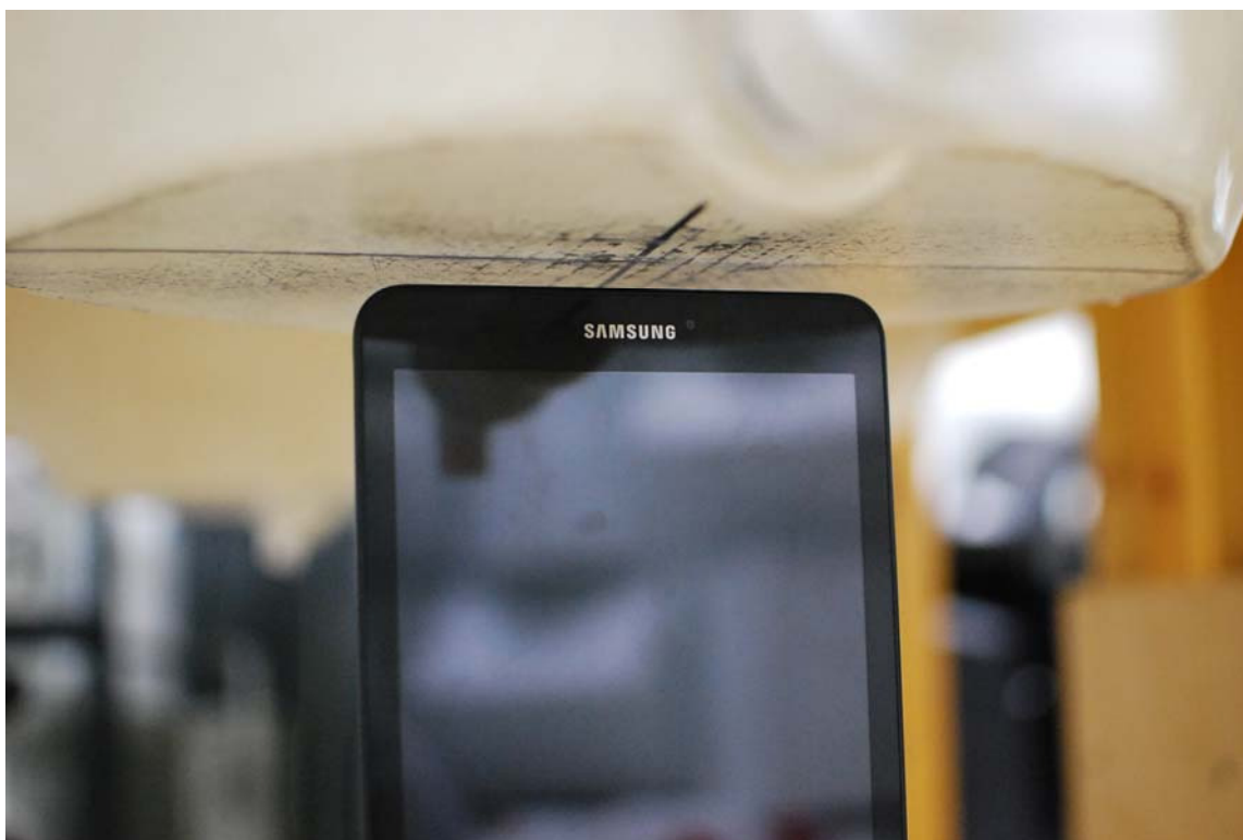
SAR Test Setup Photo 1: Top Edge at 6 mm
