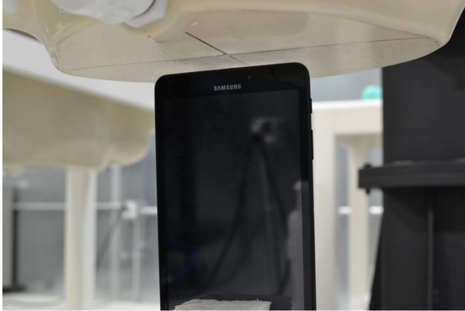
SAR Test Setup Photo 5: Top Edge at 9 mm
