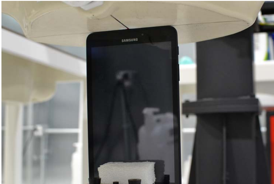
SAR Test Setup Photo 6: Top Edge at 0 mm
