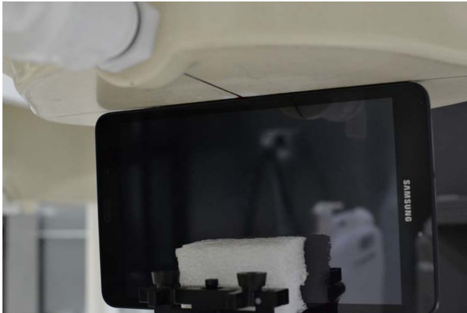
SAR Test Setup Photo 8: Left Edge at 0 mm
