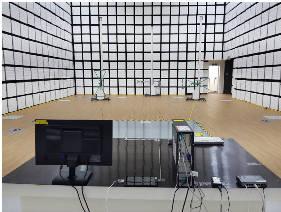
[ Radiated Disturbance for Below 1 GHz – Rear ]
