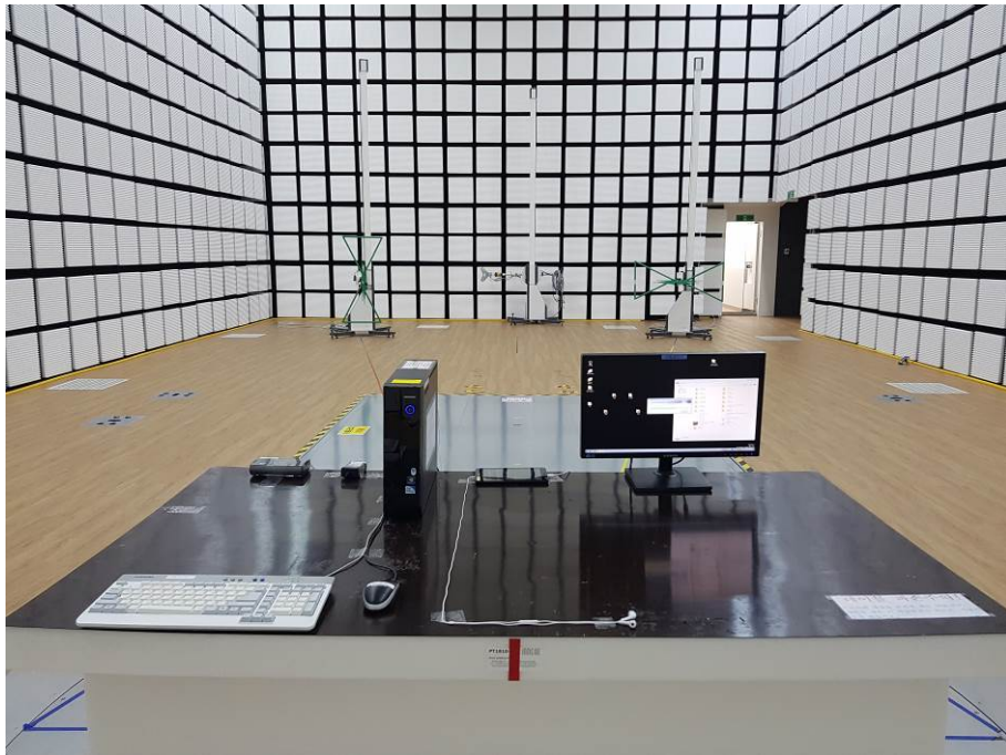
[ Radiated Disturbance for Below 1 GHz – Front ]
