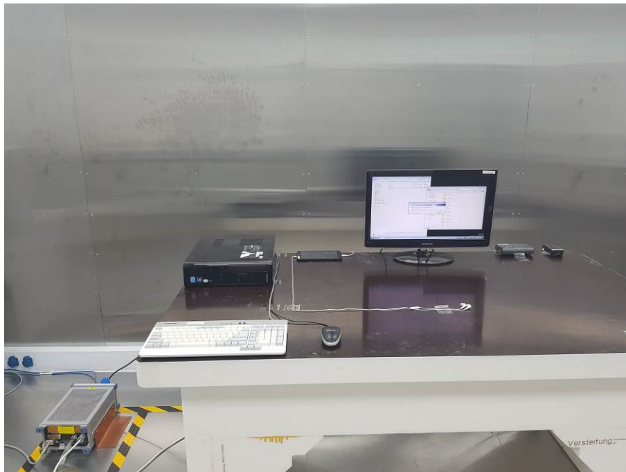
[ Conducted Disturbance – Front ]
