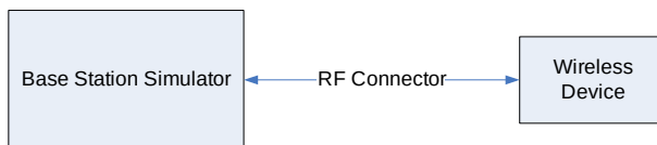
Figure 10-2 Power Measurement Setup
