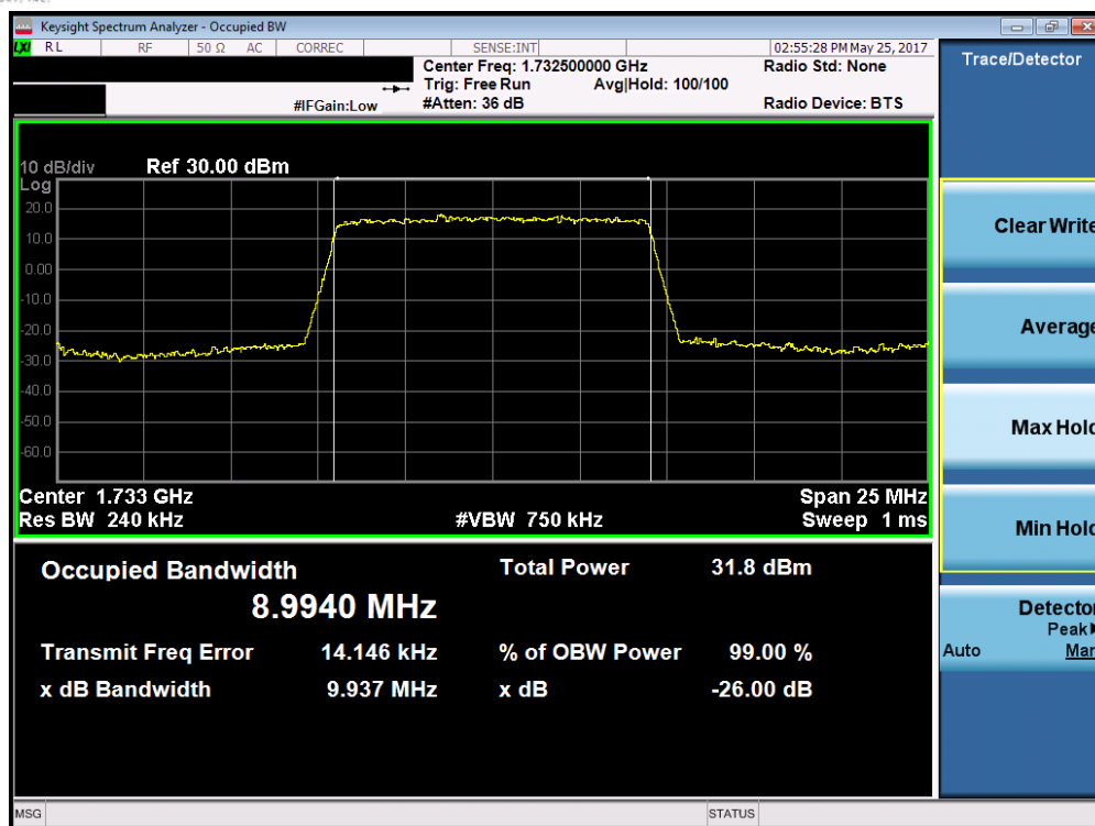
Plot 7-19. Occupied Bandwidth Plot (Band 4 – 10.0MHz QPSK – RB Size 50)
