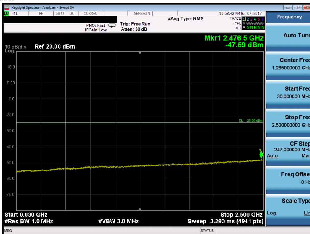
Plot 7-95. Conducted Spurious Plot (Band 7 – 5.0MHz QPSK – RB Size 1, RB Offset 0 – High Channel)
