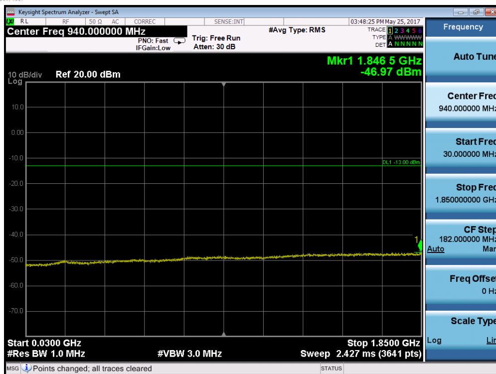
Plot 7-83. Conducted Spurious Plot (Band 2 – 10.0MHz QPSK – RB Size 1, RB Offset 0 – Mid Channel)
