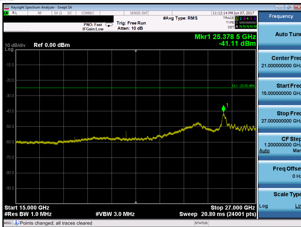
Plot 7-97. Conducted Spurious Plot (Band 7 – 5.0MHz QPSK – RB Size 1, RB Offset 0 – High Channel)
