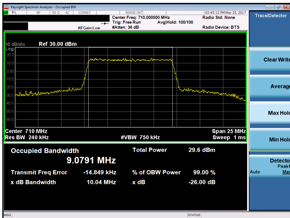
Plot 7-4. Occupied Bandwidth Plot (Band 17 – 10.0MHz 16-QAM – RB Size 50)
