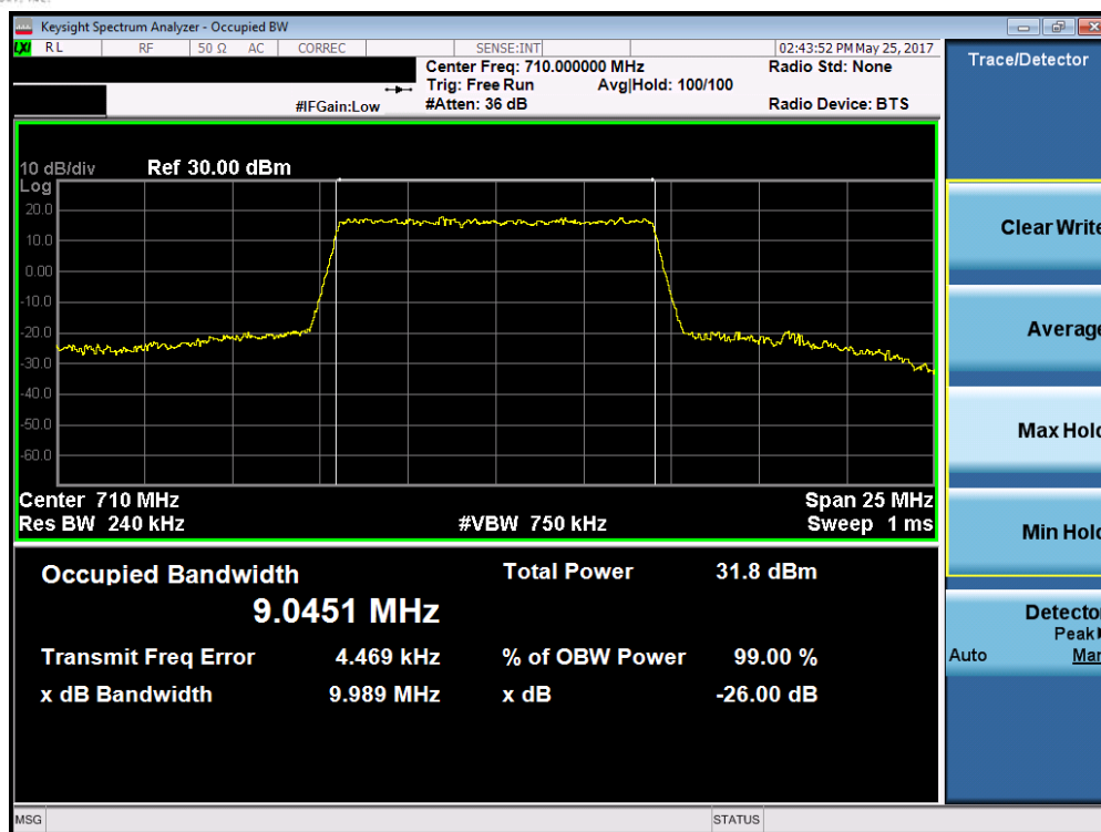
Plot 7-3. Occupied Bandwidth Plot (Band 17 – 10.0MHz QPSK – RB Size 50)
