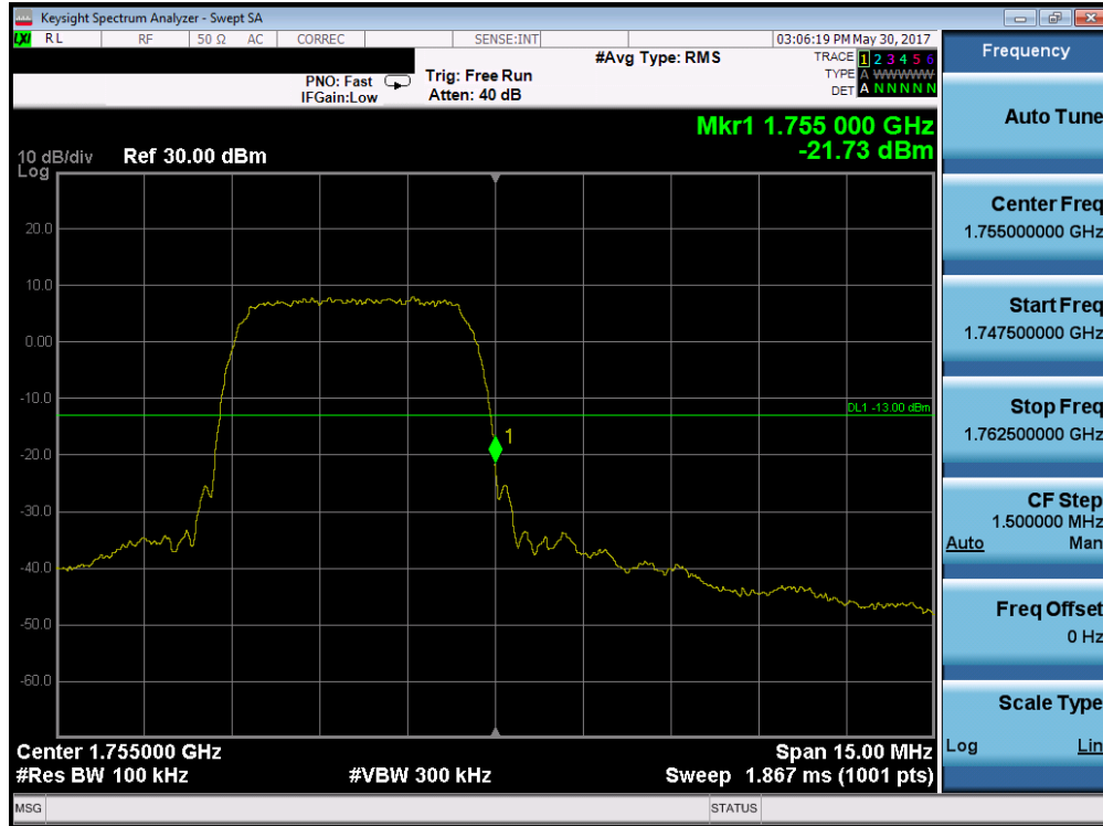
Plot 7-64. Band Edge Plot (AWS WCDMA Mode – Ch. 1513)
