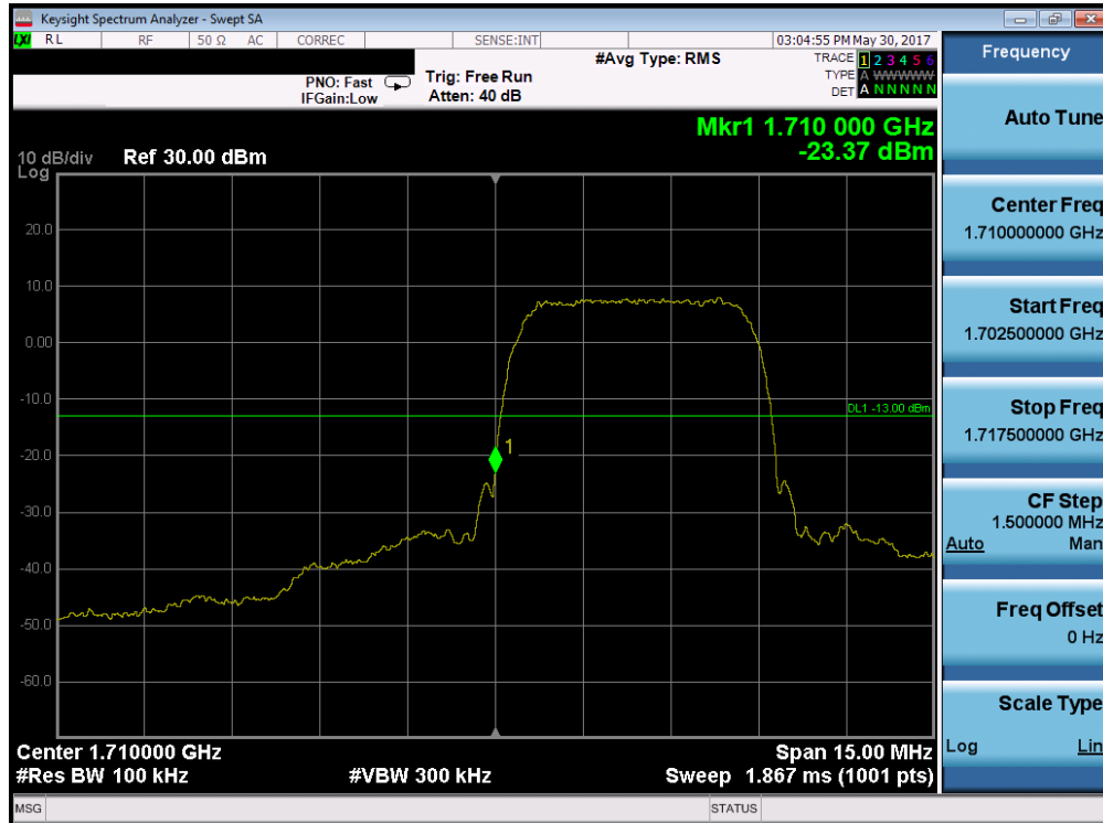
Plot 7-62. Band Edge Plot (AWS WCDMA Mode – Ch. 1312)
