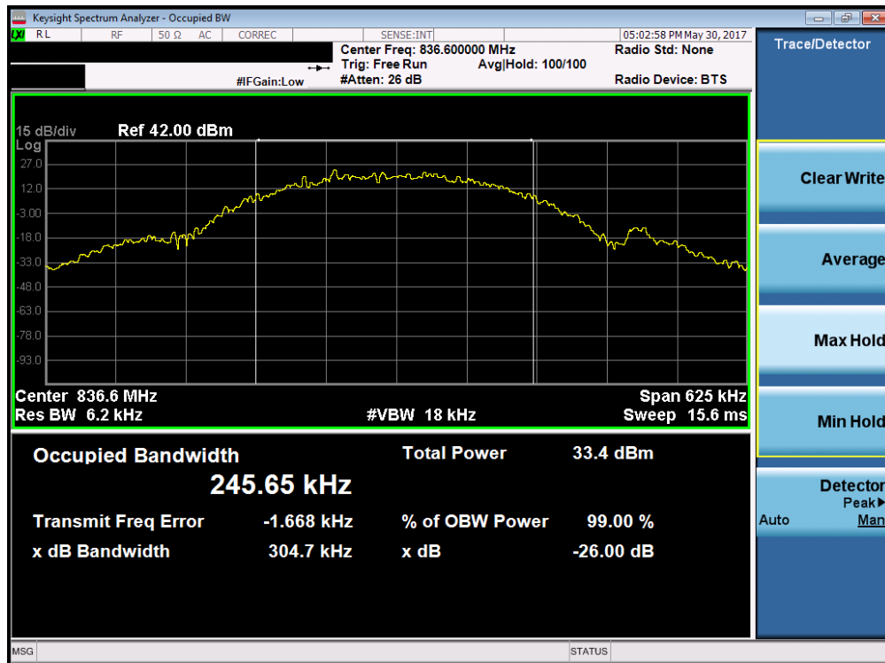
Plot 7-2. Occupied Bandwidth Plot (EDGE850 Mode – Ch. 190)
