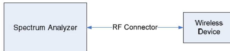
Figure 7-1. Test Instrument & Measurement Setup
