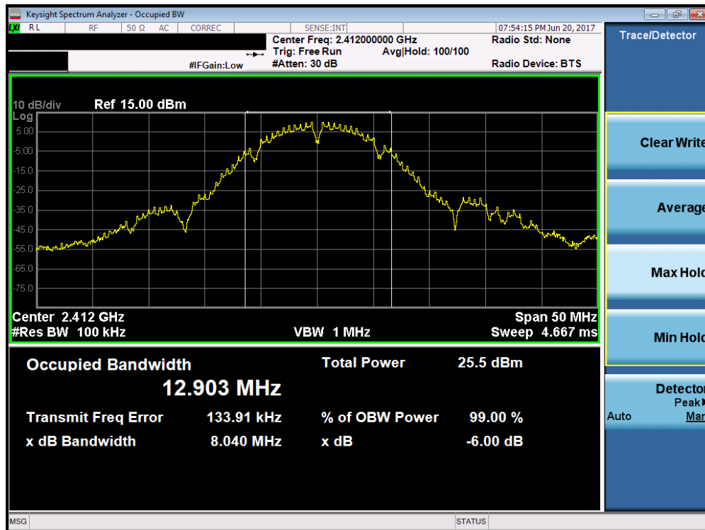
Plot 7-1. 6dB Bandwidth Plot (802.11b – Ch. 1)
