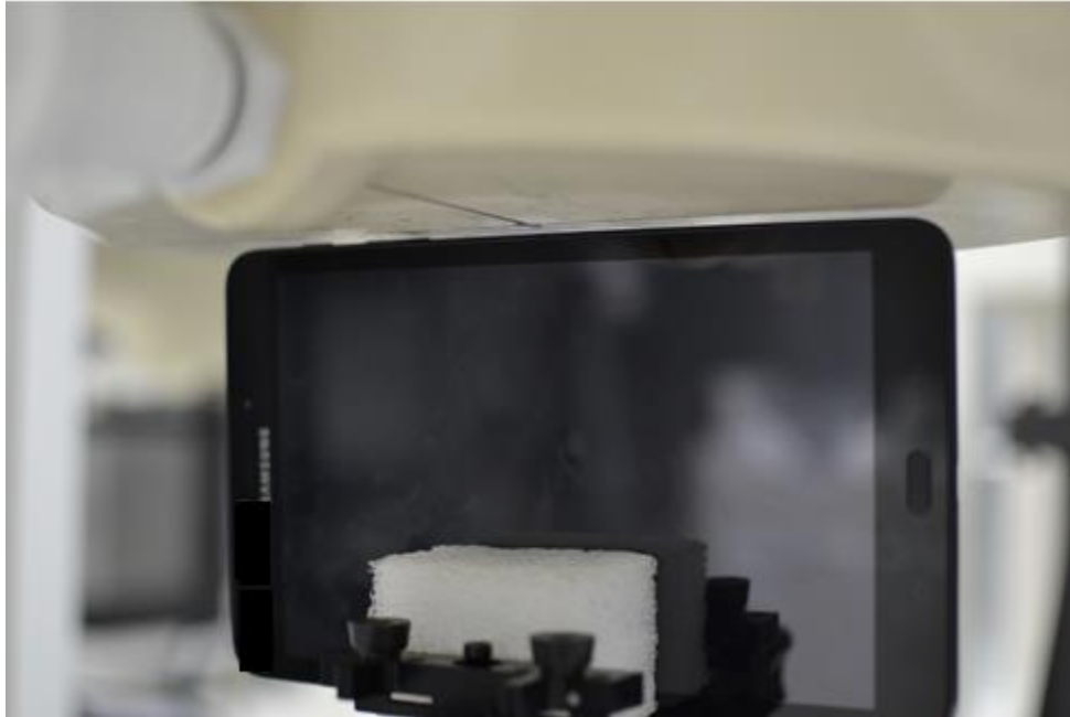
SAR Test Setup Photo 13: Right 1mm
