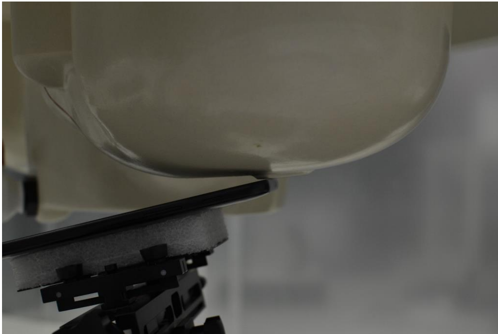
SAR Test Setup Photo 4: Left Tilt
