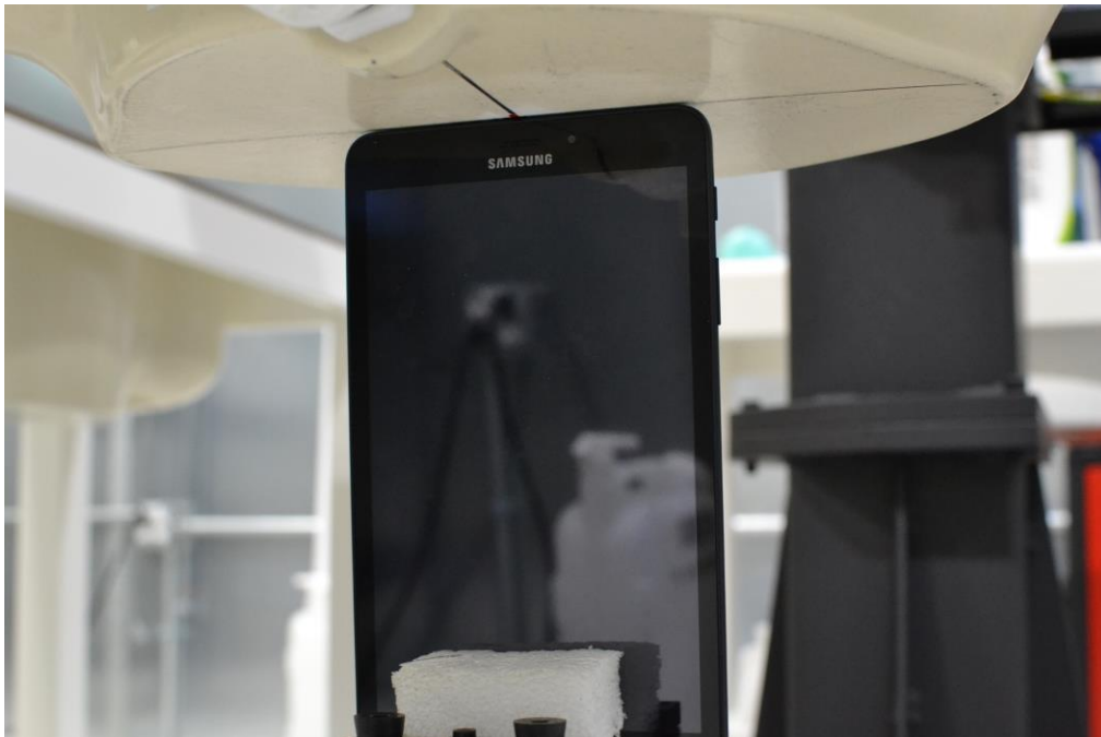
SAR Test Setup Photo 12: Top 0mm
