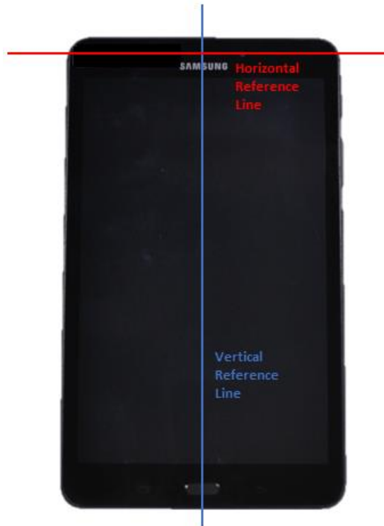
SAR Test Setup Photo 17: Vertical and Horizontal Reference Lines
