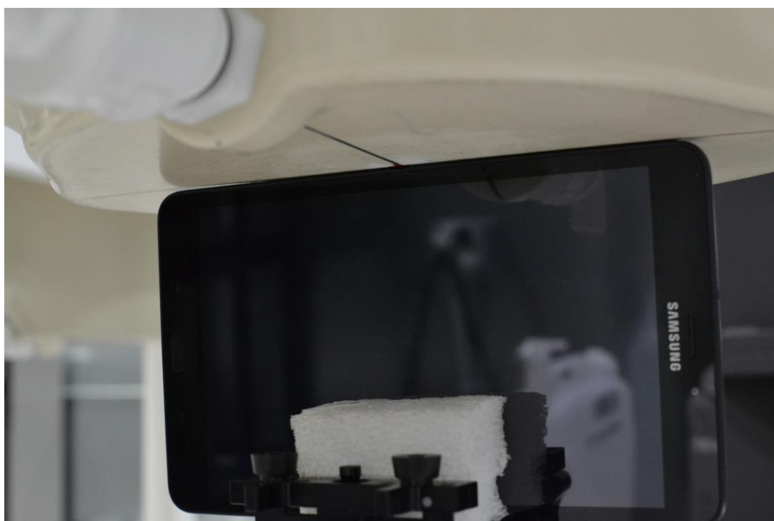
SAR Test Setup Photo 16: Left 0mm
