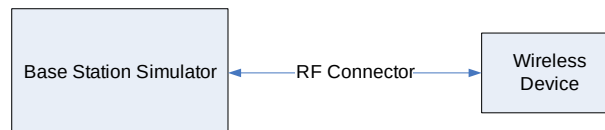
Figure 10-2 Power Measurement Setup
