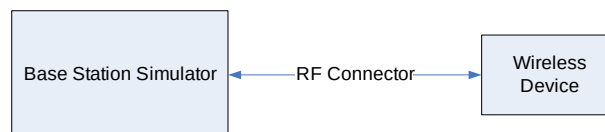
Figure 10-2 Power Measurement Setup
