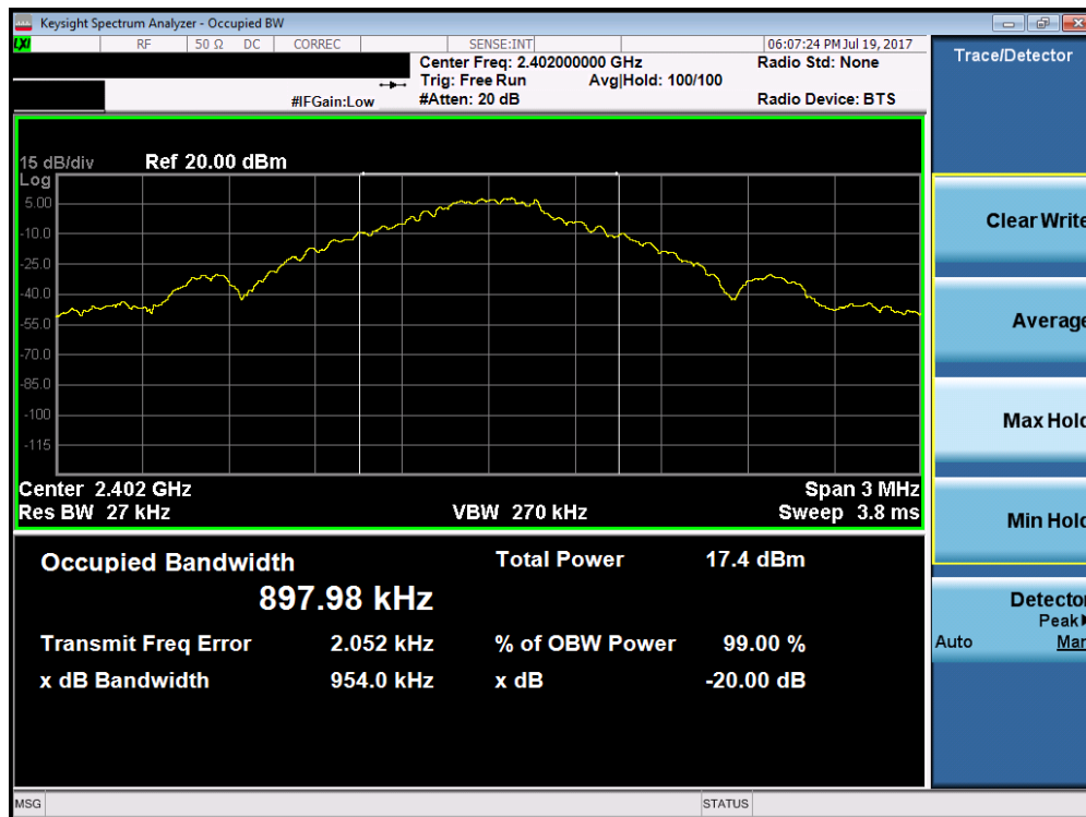
Plot 7-1. 20dB Bandwidth Plot (Bluetooth, 1Mbps – Ch. 0)
