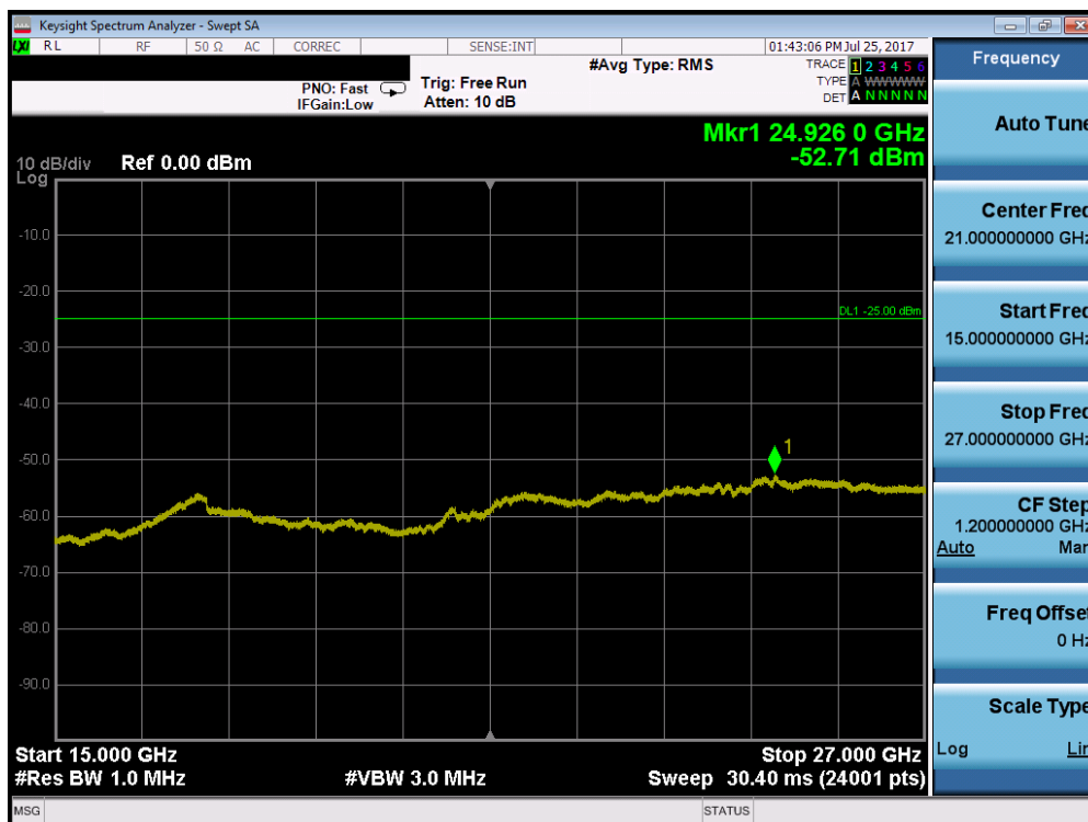
Plot 7-42. Conducted Spurious Plot (Band 7 – 5.0MHz QPSK – RB Size 1, RB Offset 0 – High Channel)
