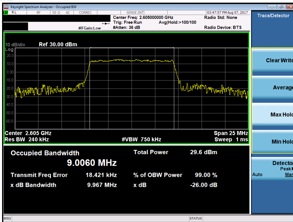
Plot 7-19. Occupied Bandwidth Plot (Band 38/41 – 10.0MHz QPSK – RB Size 50)
