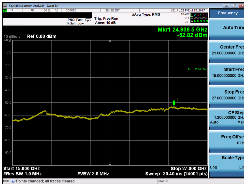
Plot 7-39. Conducted Spurious Plot (Band 7 – 5.0MHz QPSK – RB Size 1, RB Offset 0 – Mid Channel)
