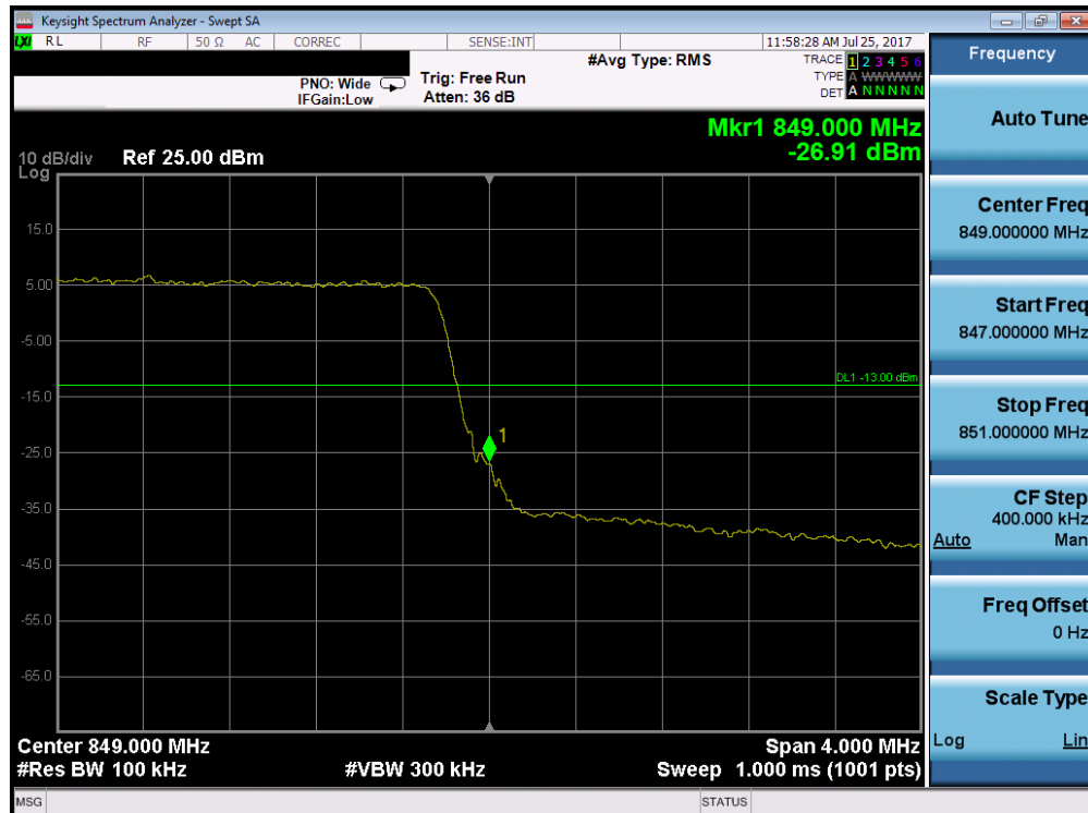
Plot 7-57. Upper Band Edge Plot (Band 5 - 5.0MHz QPSK - RB Size 25)
