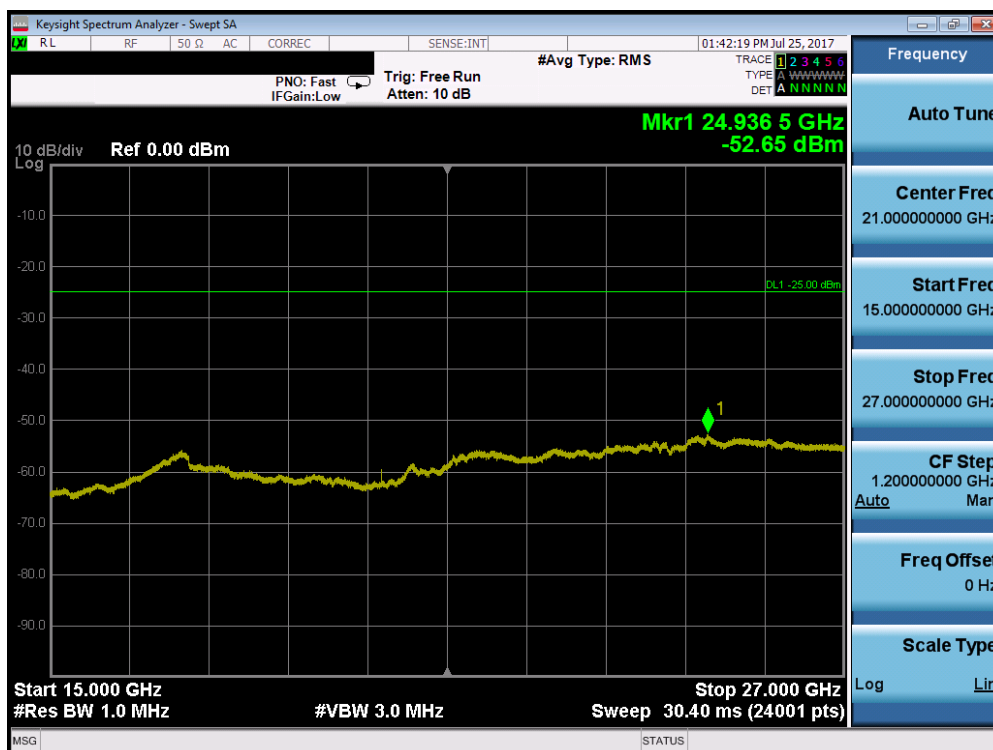
Plot 7-36. Conducted Spurious Plot (Band 7 – 5.0MHz QPSK – RB Size 1, RB Offset 0 – Low Channel)
