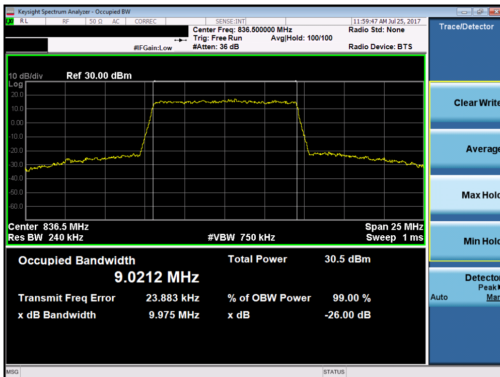
Plot 7-8. Occupied Bandwidth Plot (Band 5 – 10.0MHz 16-QAM – RB Size 50)
