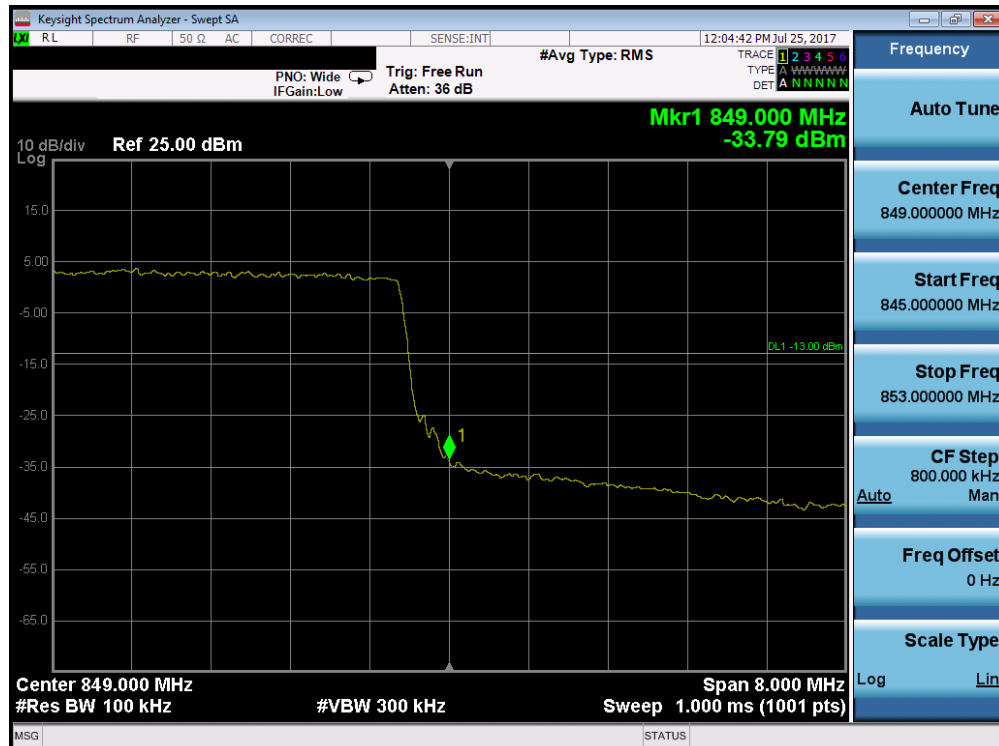
Plot 7-59. Upper Band Edge Plot (Band 5 - 10.0MHz QPSK - RB Size 50)
