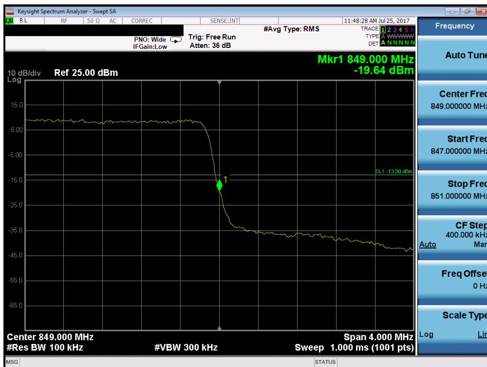
Plot 7-55. Upper Band Edge Plot (Band 5 - 3.0MHz QPSK - RB Size 15)
