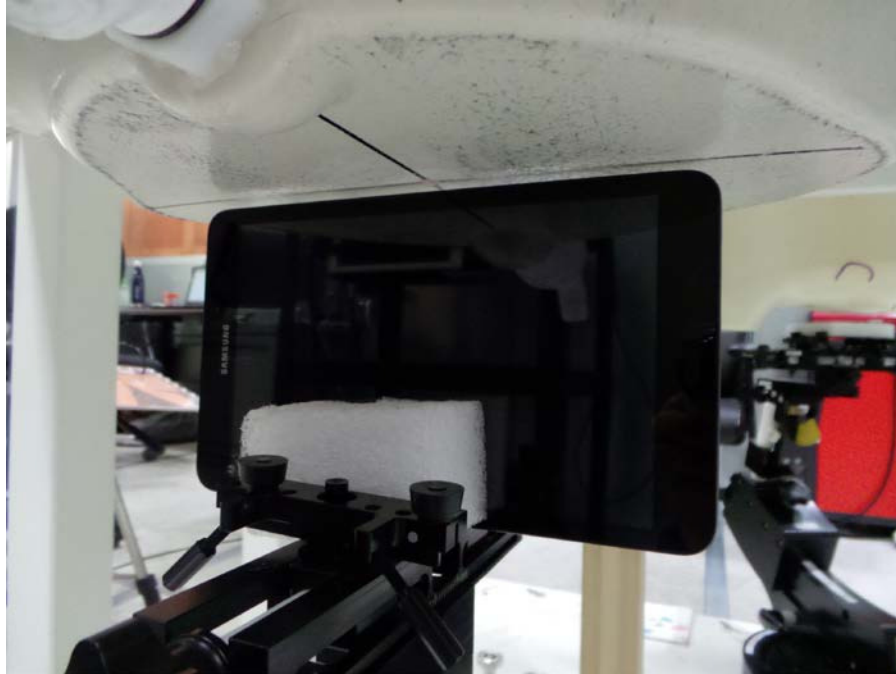
SAR Test Setup Photo 13: Right 1mm
