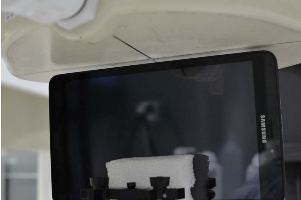
SAR Test Setup Photo 15: Left 3mm
