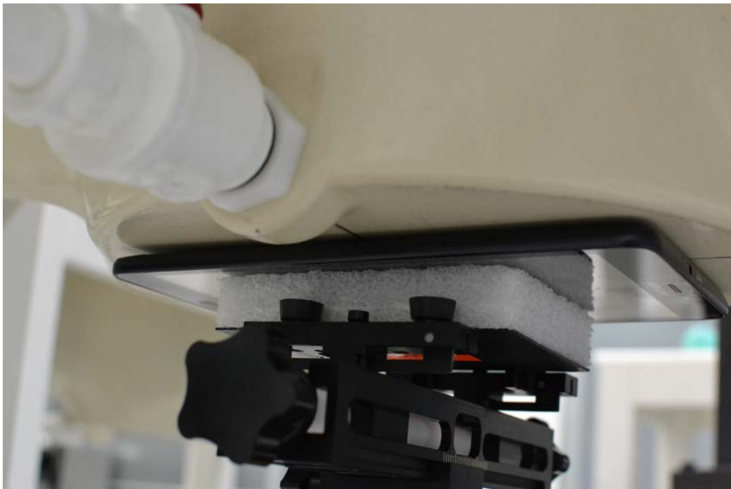
SAR Test Setup Photo 8: Back 0 mm
