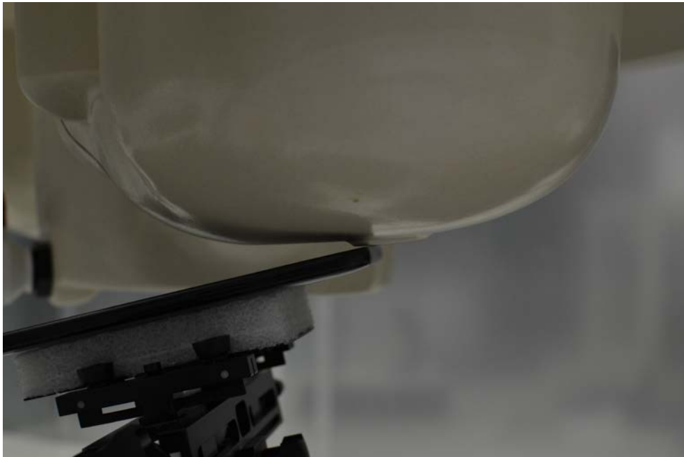
SAR Test Setup Photo 4: Left Tilt
