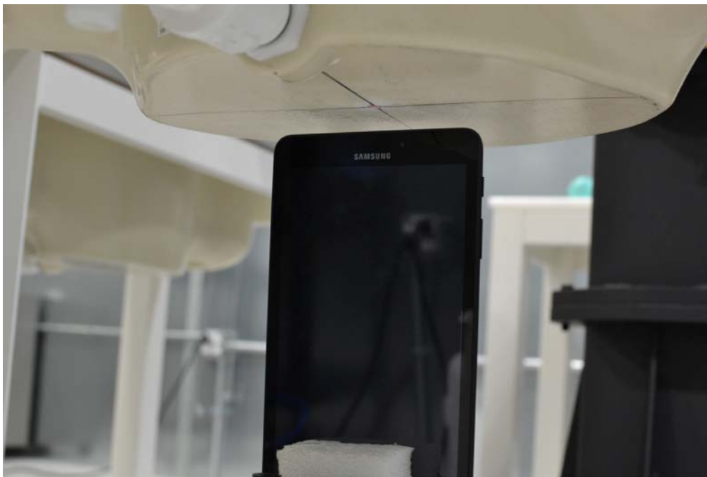
SAR Test Setup Photo 10: Top 14mm
