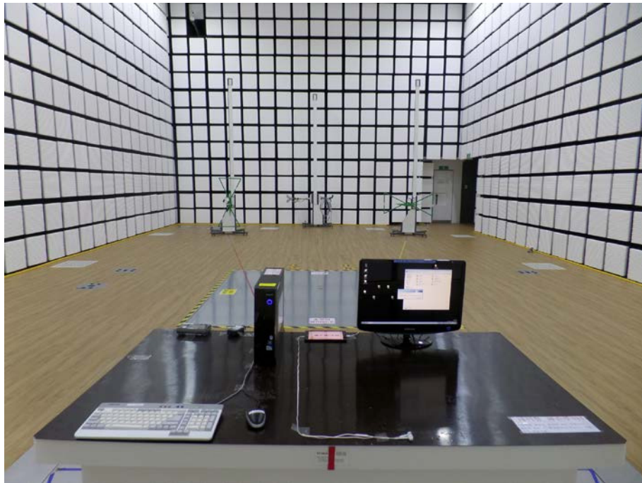
[ Radiated Disturbance for Below 1 GHz – Front ]
