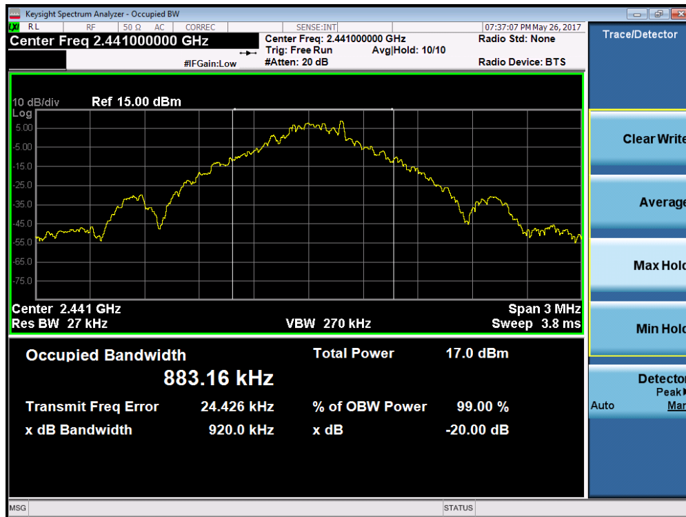
Plot 7-2. 20dB Bandwidth Plot (Bluetooth, 1Mbps – Ch. 39)
