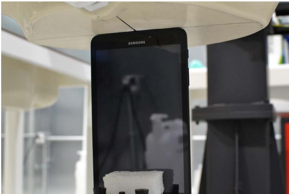
SAR Test Setup Photo 12: Top 0mm
