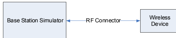
Figure 10-2 Power Measurement Setup
