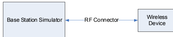
Figure 10-1 Power Measurement Setup
