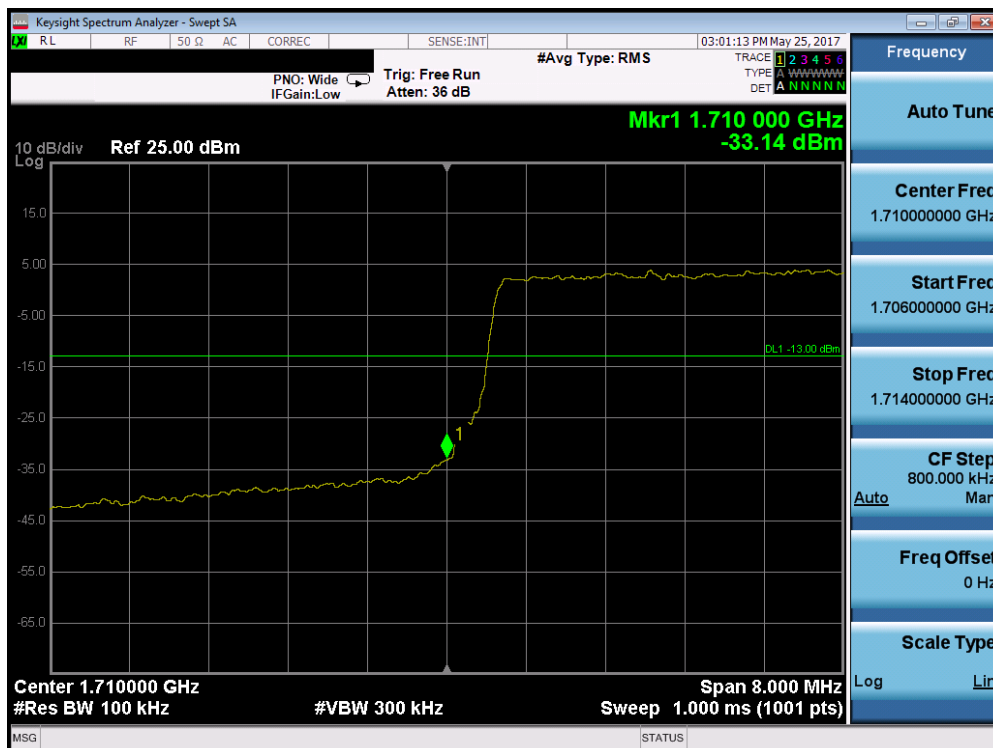
Plot 7-123. Lower Band Edge Plot (Band 4 – 10.0MHz QPSK – RB Size 50)
