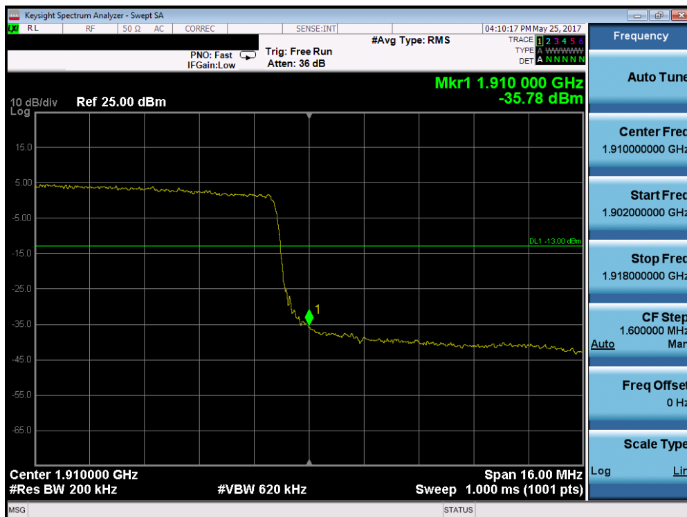
Plot 7-181. Upper Band Edge Plot (Band 2 – 20.0MHz QPSK – RB Size 100)
