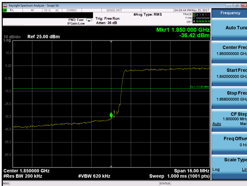
Plot 7-179. Lower Band Edge Plot (Band 2 – 20.0MHz QPSK – RB Size 100)
