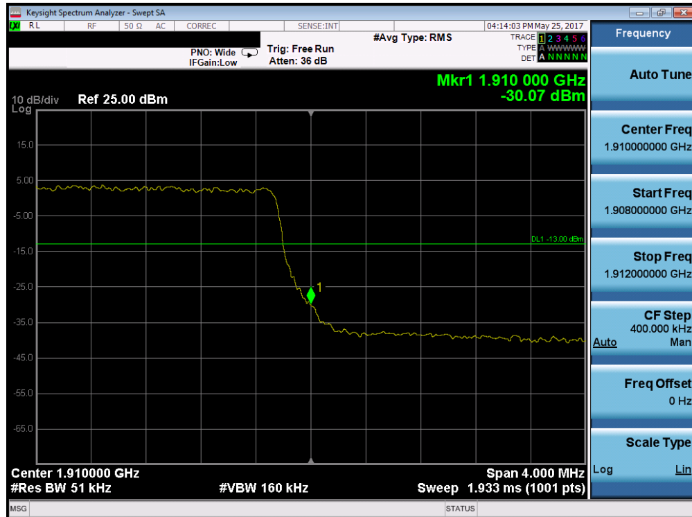
Plot 7-169. Upper Band Edge Plot (Band 2 – 5.0MHz QPSK – RB Size 25)
