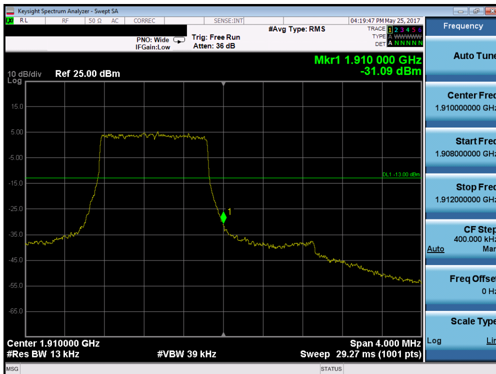
Plot 7-161. Upper Band Edge Plot (Band 2 – 1.4MHz QPSK – RB Size 6)
