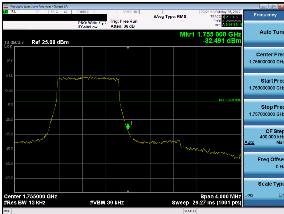
Plot 7-113. Upper Band Edge Plot (Band 4 – 1.4MHz QPSK – RB Size 6)
