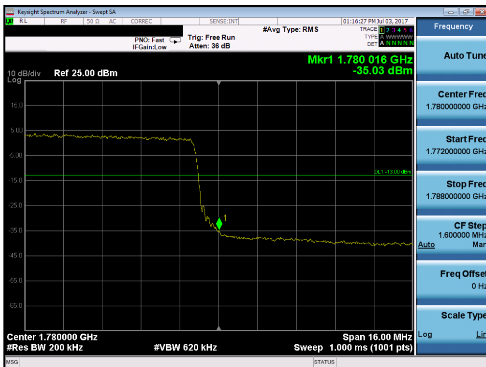
Plot 7-157. Upper Band Edge Plot (Band 66 – 20.0MHz QPSK – RB Size 100)
