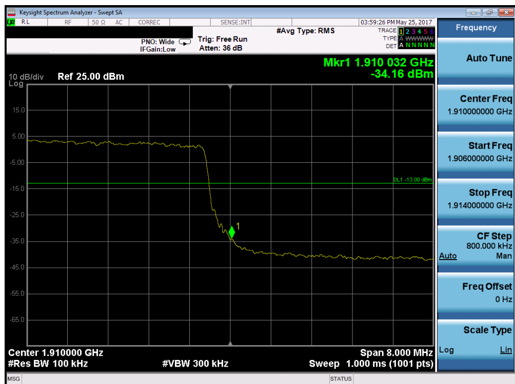
Plot 7-173. Upper Band Edge Plot (Band 2 – 10.0MHz QPSK – RB Size 50)
