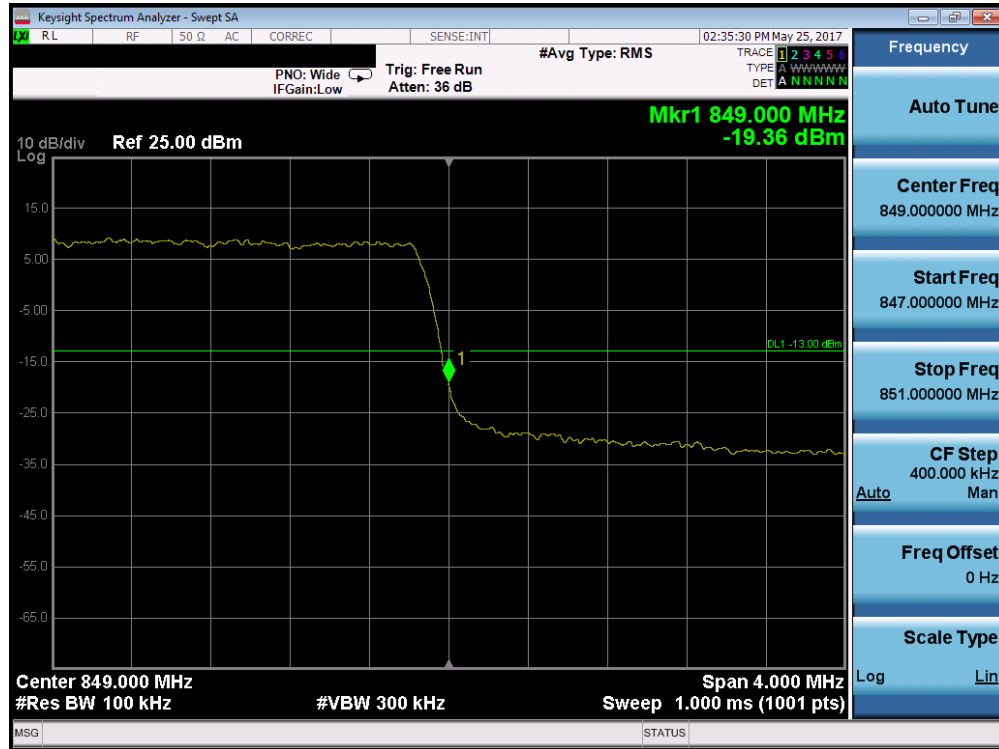
Plot 7-106. Upper Band Edge Plot (Band 5 - 3.0MHz QPSK - RB Size 15)
