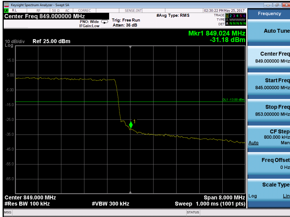
Plot 7-110. Upper Band Edge Plot (Band 5 – 10.0MHz QPSK – RB Size 50)
