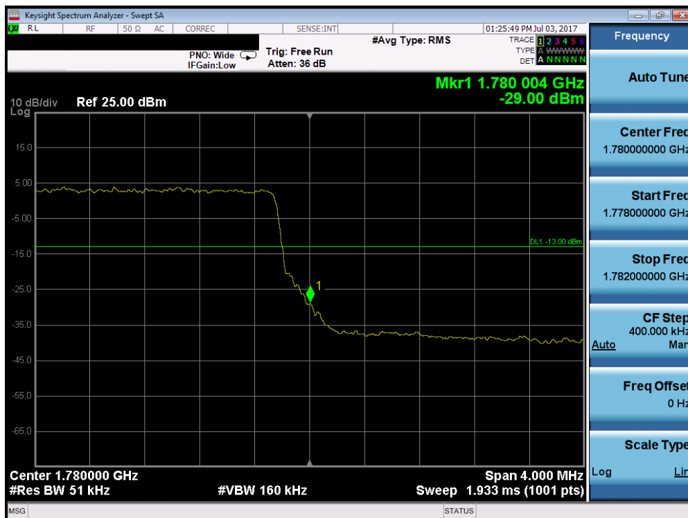
Plot 7-145. Upper Band Edge Plot (Band 66 – 5.0MHz QPSK – RB Size 25)
