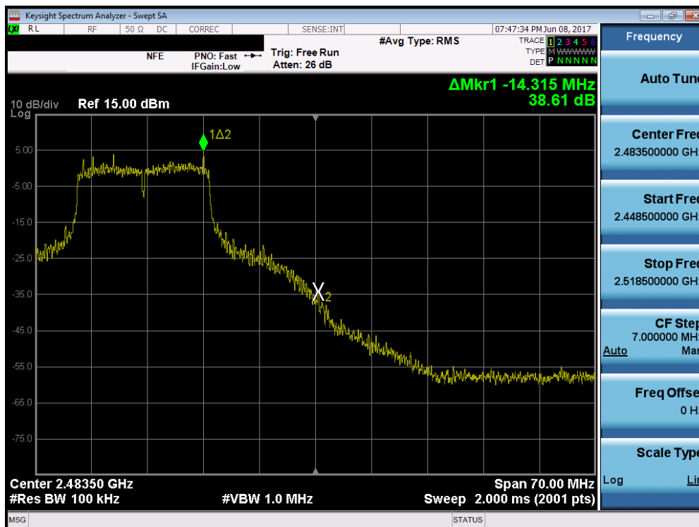
Plot 7-22. Band Edge Plot (802.11g – Ch. 11)
