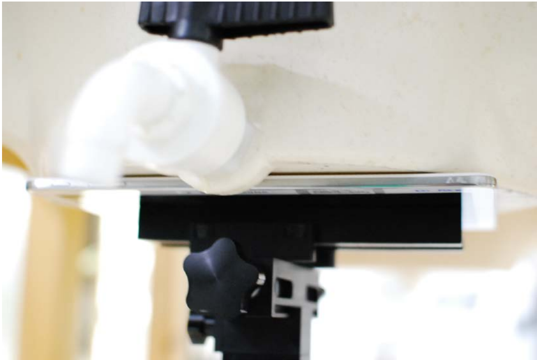
SAR Test Setup Photo 1: Back at 0.0 mm
