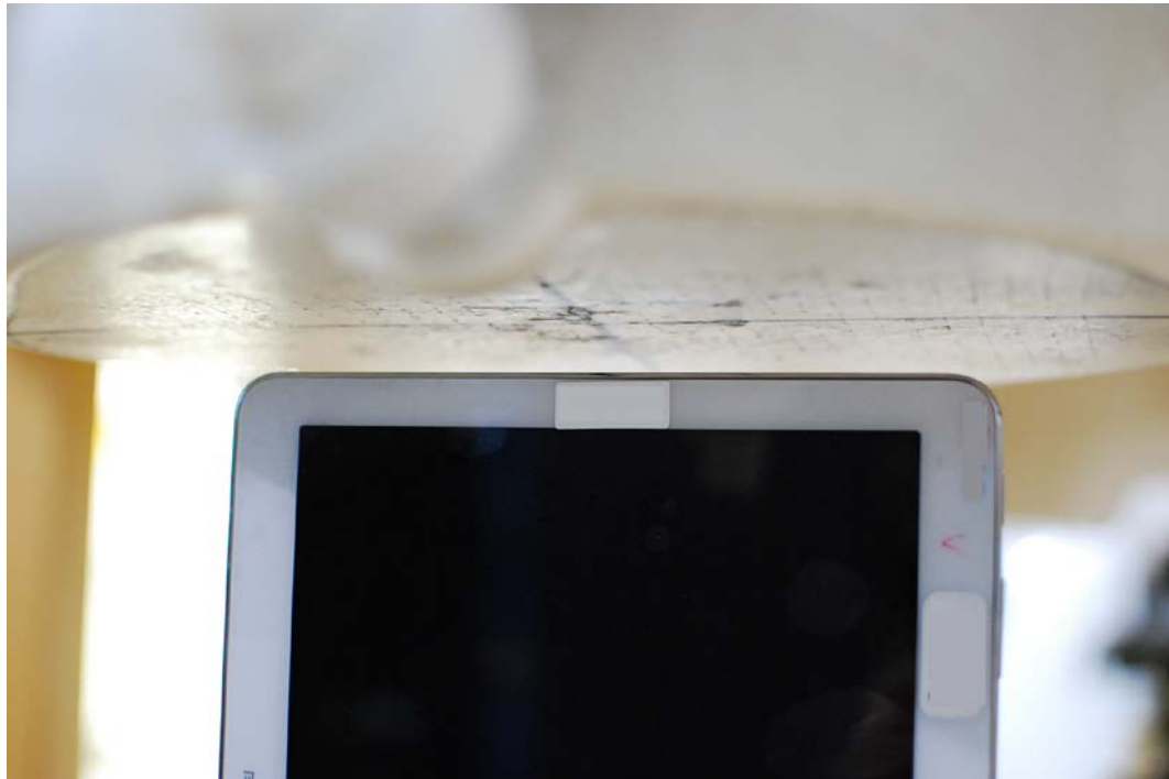
SAR Test Setup Photo 5: Left at 15 mm
