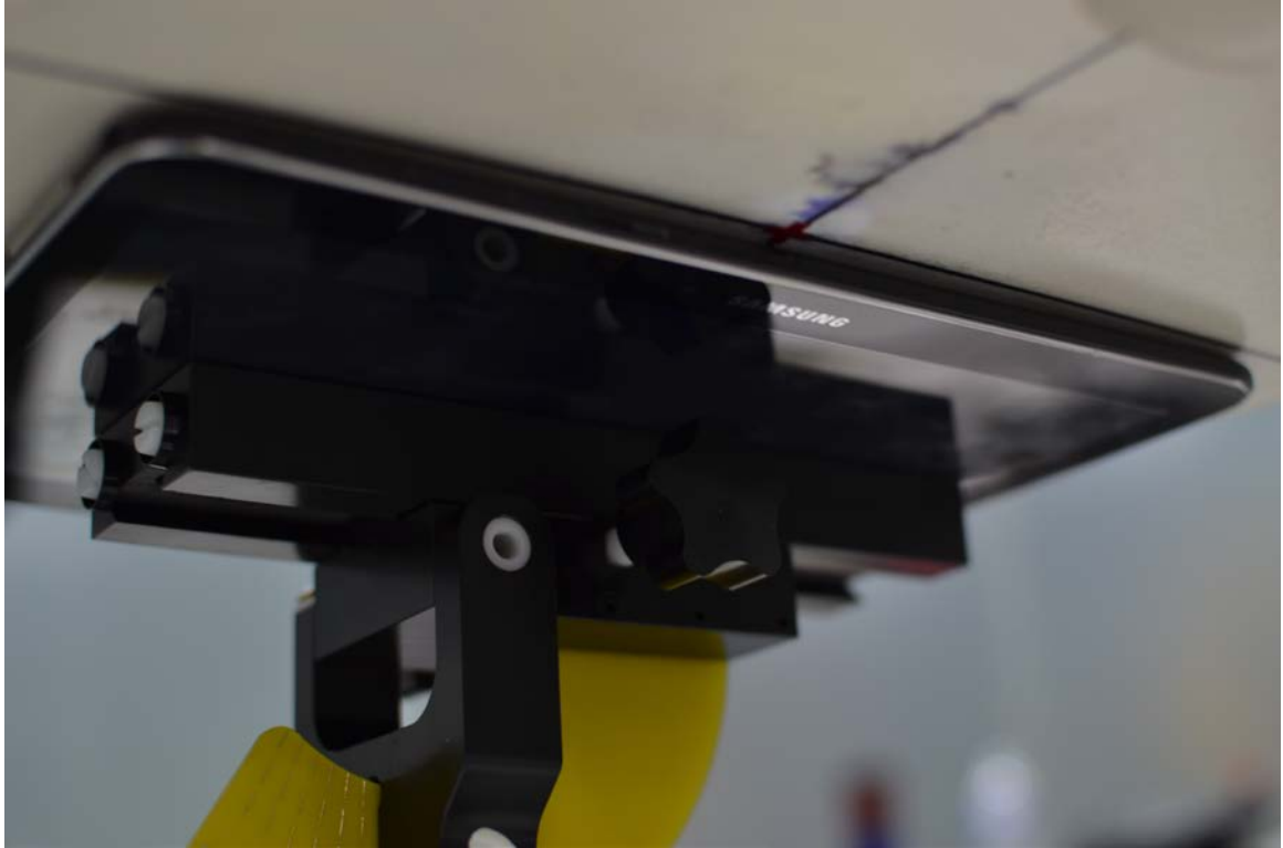
SAR Test Setup Photo 1: Back Side at 0.0 cm
