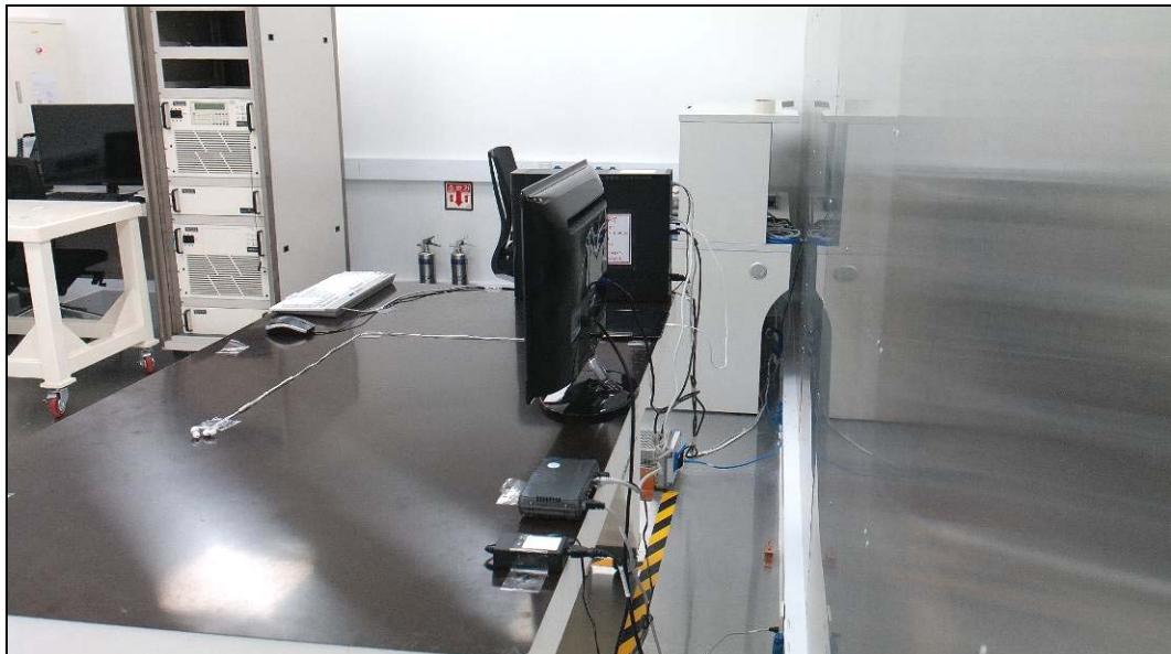
[ Conducted Disturbance – Rear ]
