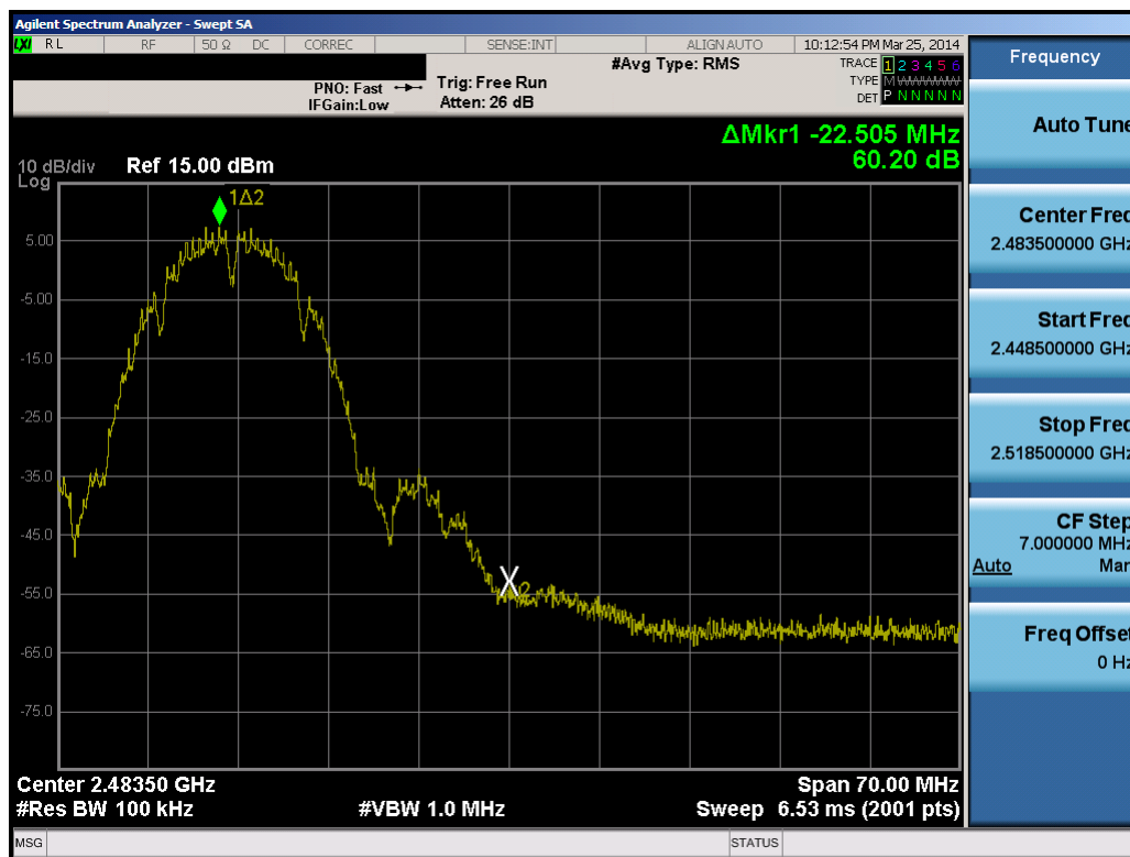
Plot 6-36. Band Edge Plot (802.11b – Ch. 11)
