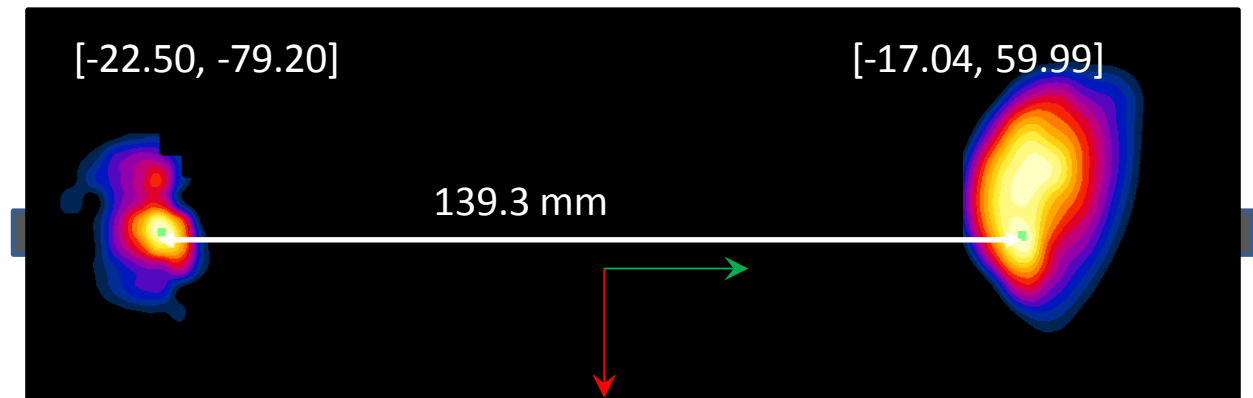
Figure 11-19 Peak SAR Locations for Body Top Edge at 22 mm LTE B2 and 2.4 GHz WLAN Antenna
